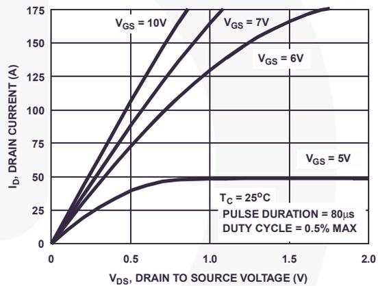
**Figure 8. Saturation Characteristics**
