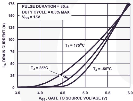
**Figure 7. Transfer Characteristics**
