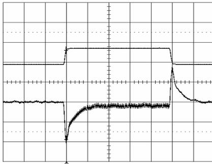
Output voltage response to load current step-
