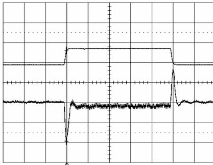
Output voltage response to load current step-
