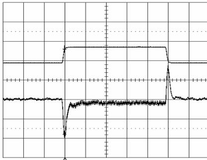
Output voltage response to load current step-
