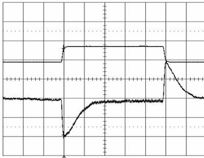
Output voltage response to load current step-
