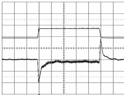
Output voltage response to load current step-
