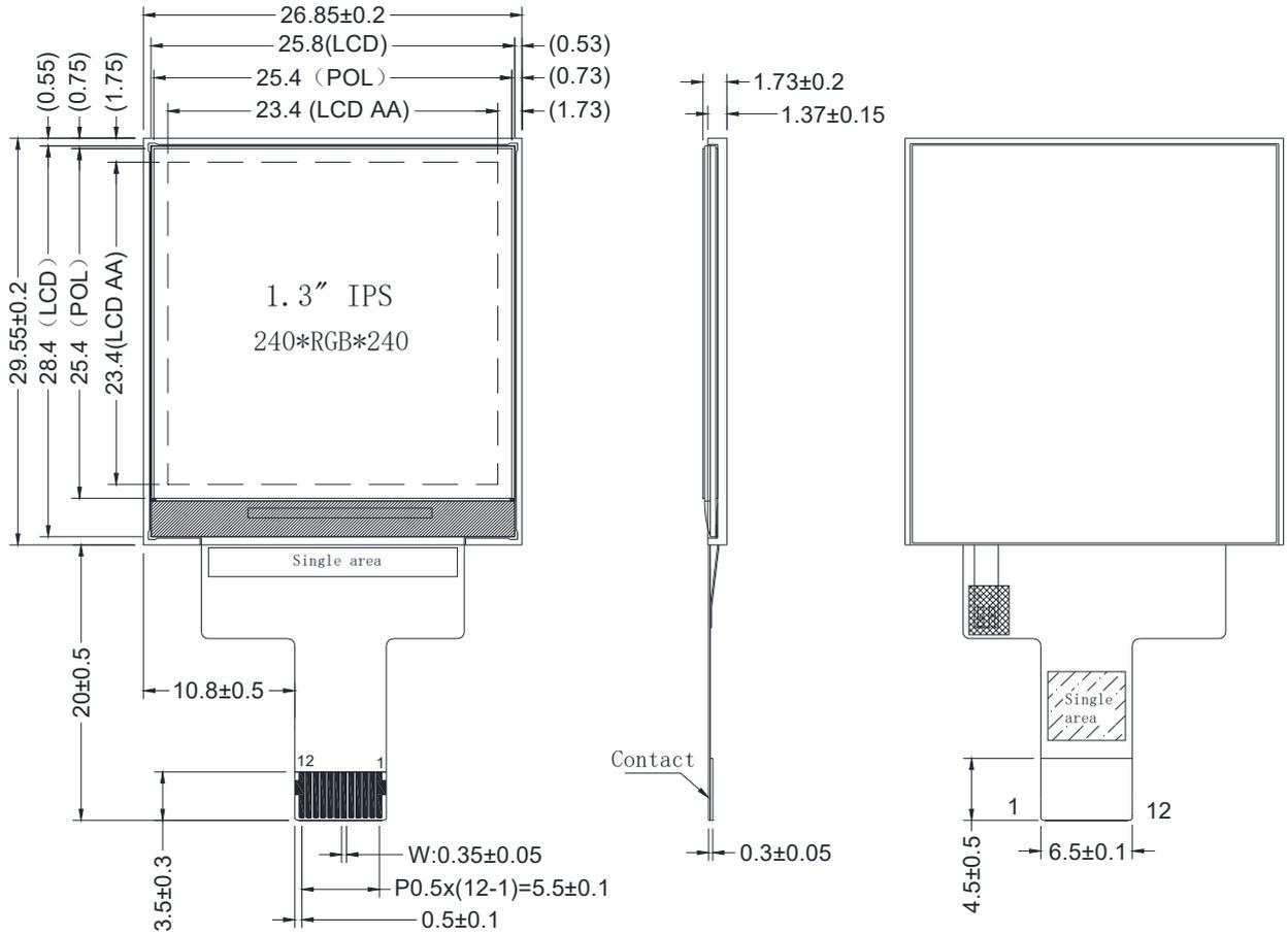
1. Unspecifide tolerance:  $\pm 0.3\text{mm}$
