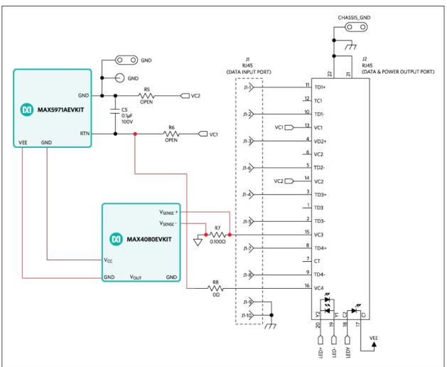
Figure 2. MAX5971A and MAX4080 EV kits and current sense resistor R7 connections.
