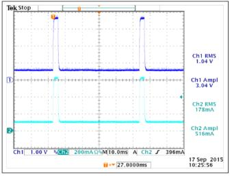
Figure 3. 100mA DC and 600mA transient current loading at 20Hz, 10% duty cycle.
