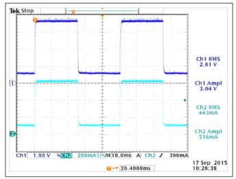
Figure 5. 100mA DC and 600mA transient current loading at 20Hz, 50% duty cycle.
