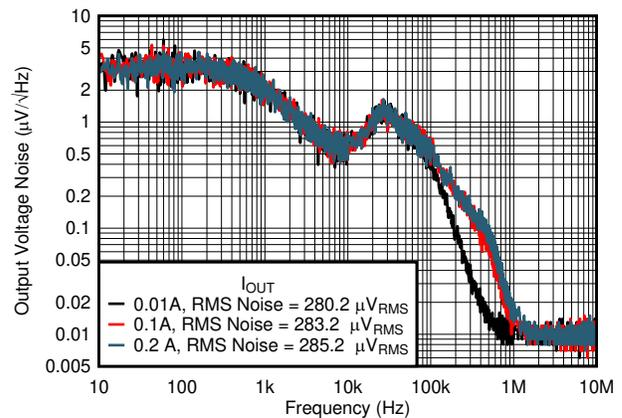
$V_{OUT} = 1.24\text{ V}$ ,  $C_{IN} = 1\ \mu\text{F}$ ,  $C_{OUT} = 1\ \mu\text{F}$ ,  $C_{FF} = 10\text{ nF}$ ,  $V_{RMS}$
