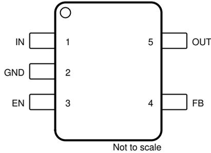
**Figure 5-1. DBV Package (Adjustable), 5-Pin SOT-23 (Top View)**
