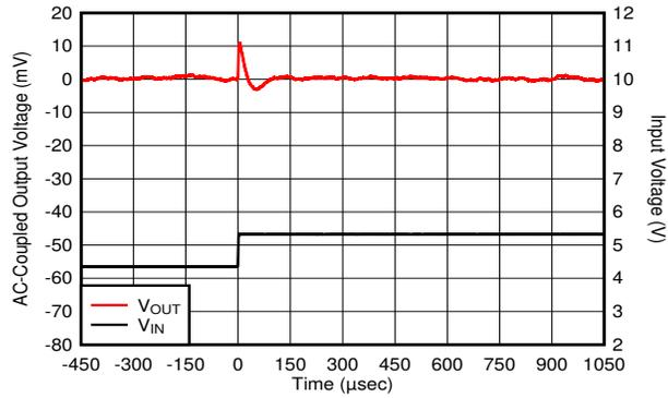
**Figure 8-5. Line Transient (4.3 V to 5.3 V)**
