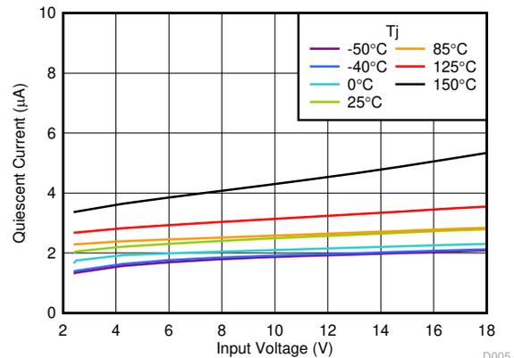
Figure 6-10.  $I_Q$  vs  $V_{IN}$
