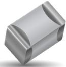
AVX has developed a range of multilayer ceramic capacitors designed for use in applications up to 150°C. These capacitors are manufactured with an X8R and an X8L dielectric material. X8R material has capacitance variation of ± 15% between -55°C and +150°C. The X8L material has capacitance variation of ±15% between -55°C to 125°C to 125°C and +15/40% from +125°C to +150°C.
