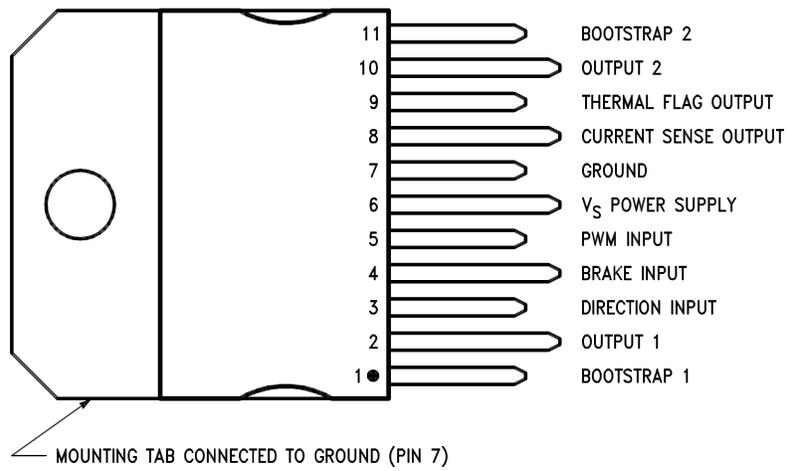
**Figure 2. 11-Lead TO-220 Package
