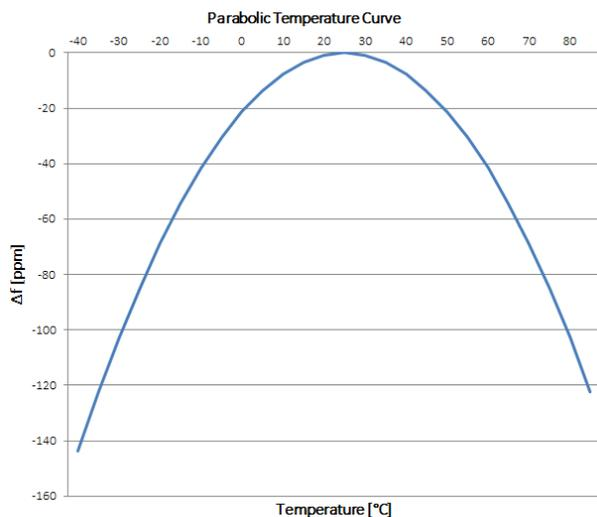
Frequency Stability [ $\Delta f$ ] at a given temperature,
