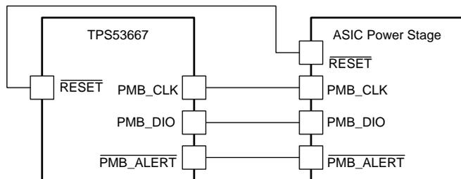
Figure 17. RESET Pin Connection
