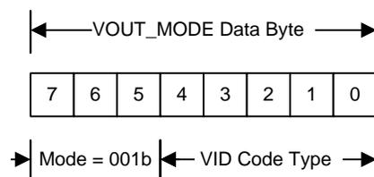
Figure 21. VOUT\_MODE Data Byte for VID Mode
