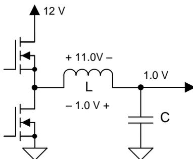
Figure 12. Representative Schematic of Synchronous Buck Converter Circuit
