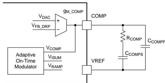
Figure 106. Compensation Circuitry
