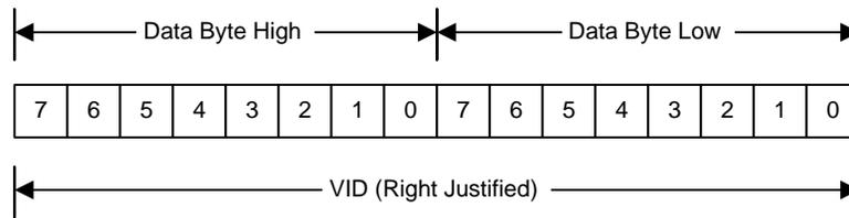
**Figure 22. VOUT\_COMMAND Data Bytes for VID Mode**
