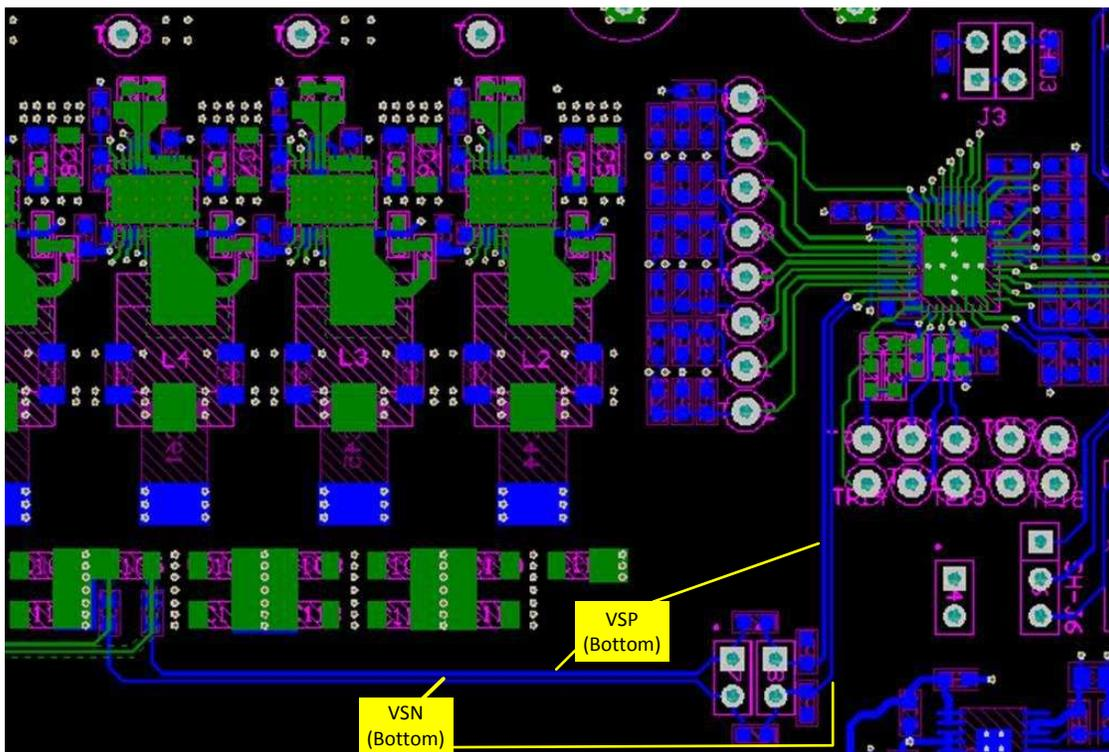
Figure 125. Layout Example for Feedback Voltage Sensing Traces
