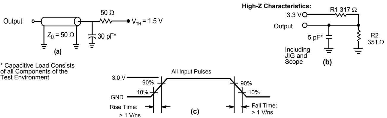
\* Capacitive Load Consists of all Components of the Test Environment
