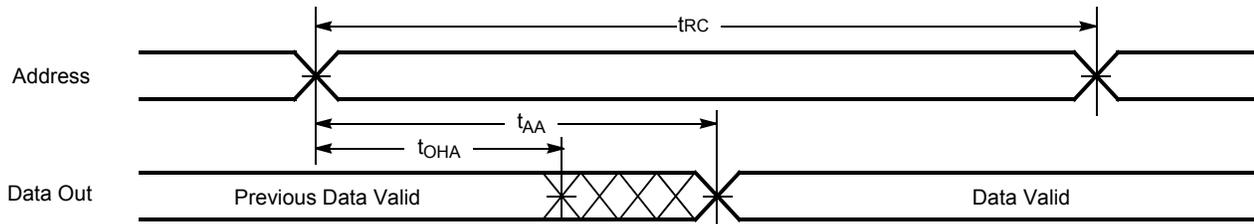
Figure 8. Read Cycle No. 2 ( $\overline{OE}$  Controlled) [18, 19, 20]
