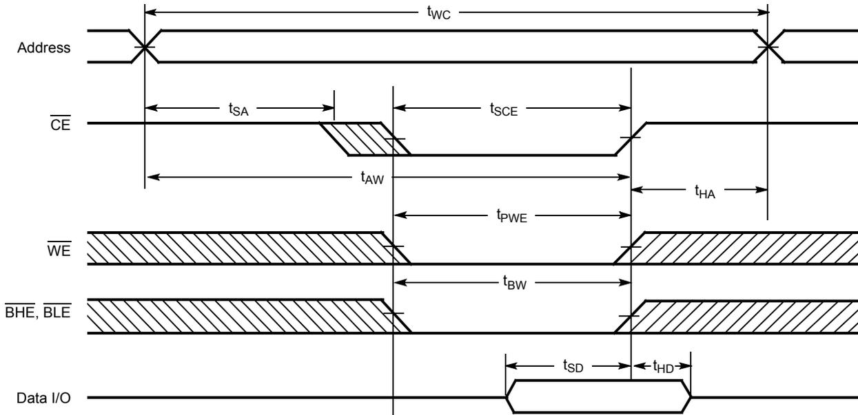
Figure 10. Write Cycle No. 2 ( $\overline{\text{WE}}$  Controlled,  $\overline{\text{OE}}$  LOW) [21, 22, 23, 24]
