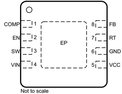
Figure 5-2. NGT Package 8-Pin WSON Top View
