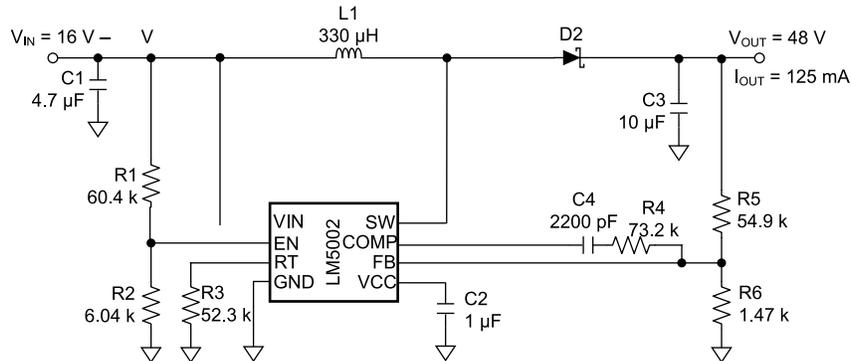
Figure 8-7. Boost Schematic
