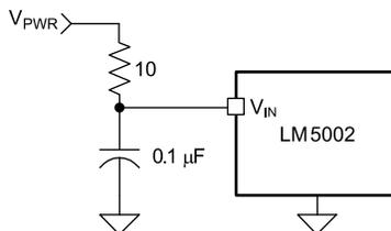
**Figure 8-1. Input Transient Protection**
