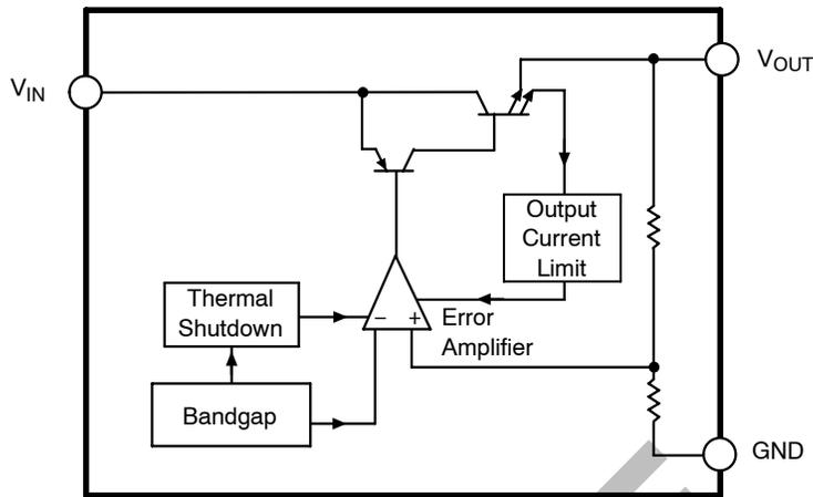
Figure 2. Block Diagram – CS5205-3, -5
