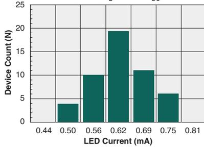
**Typical  $I_L$  for Switch Dropout**
