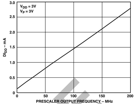
TPC 22. DI<sub>DD</sub> vs. Prescaler Output Frequency (ADF4218, RF Only)
