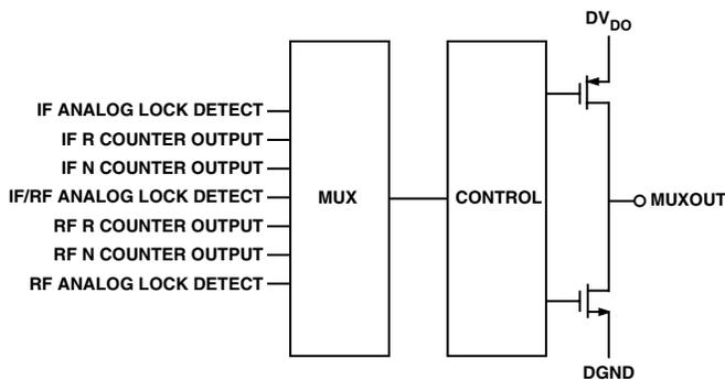
Figure 6. MUXOUT Circuit
