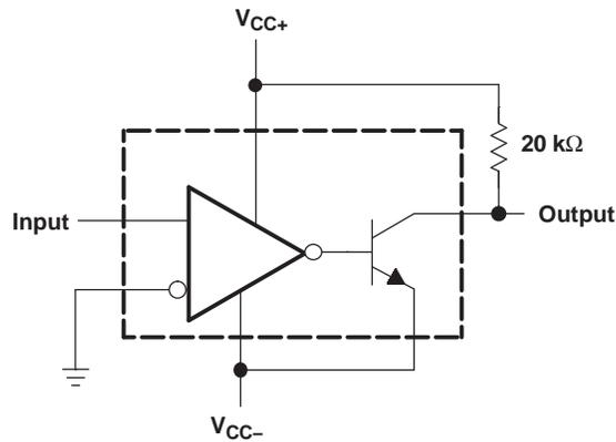
Figure 14. Zero-Crossing Detector
