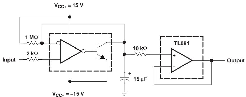
Figure 25. Negative-Peak Detector
