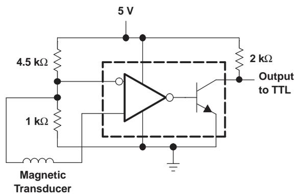
Figure 16. Detector for Magnetic Transducer
