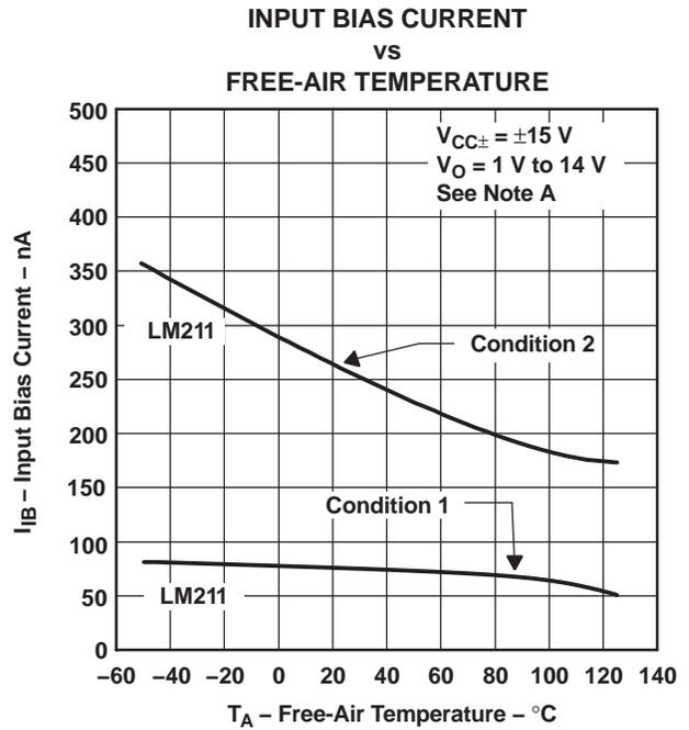
NOTE A: Condition 1 is with BALANCE and BAL/STRB open. Condition 2 is with BALANCE and BAL/STRB connected to V<sub>CC+</sub>.
