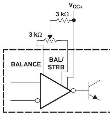
NOTE: If offset balancing is not used, the BALANCE and BAL/STRB pins should be shorted together.
