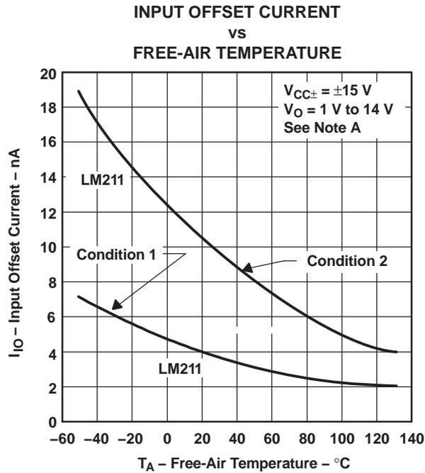
NOTE A: Condition 1 is with BALANCE and BAL/STRB open. Condition 2 is with BALANCE and BAL/STRB connected to V<sub>CC+</sub>.
