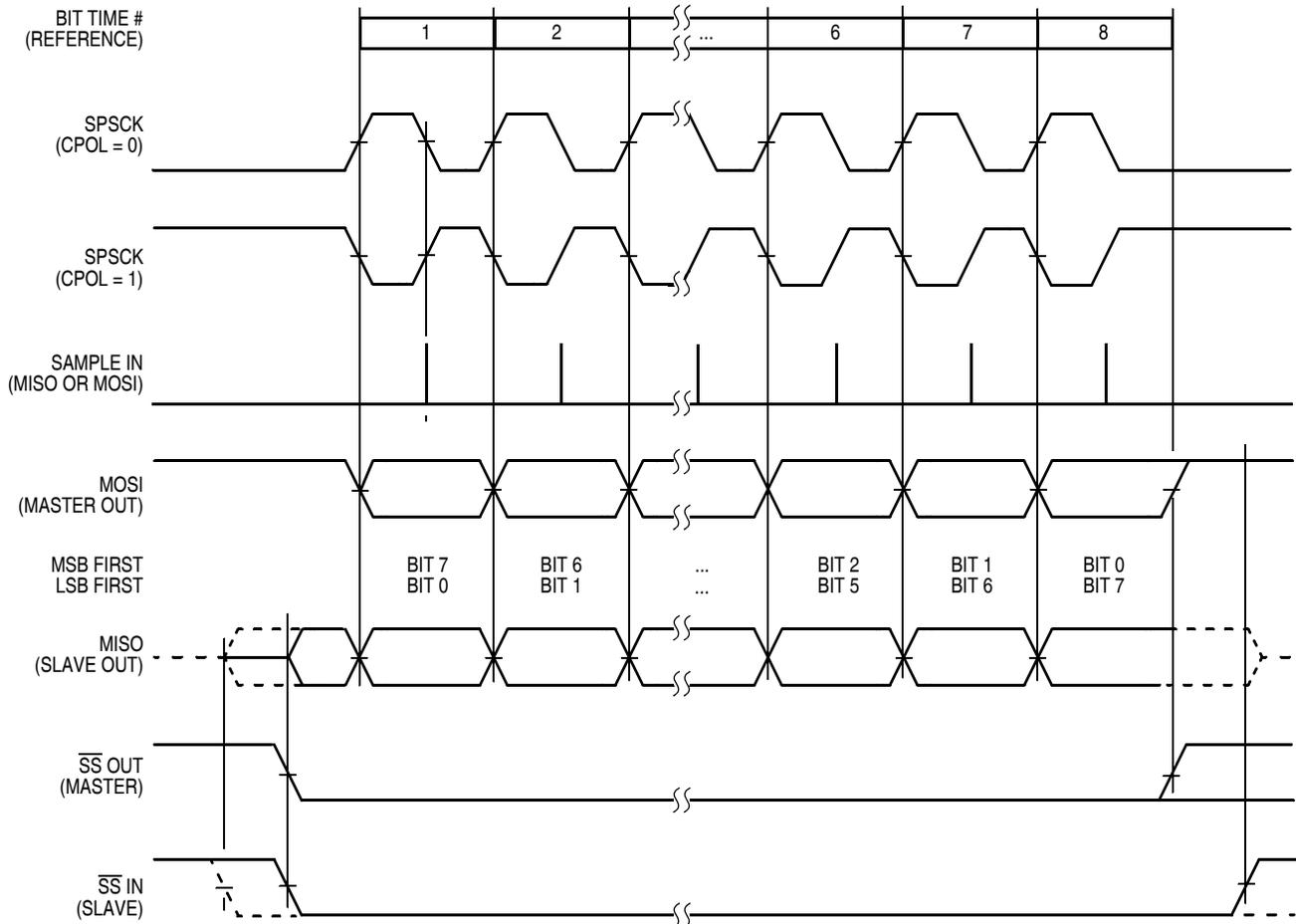
**Figure 12-10. SPI Clock Formats (CPHA = 1)**
