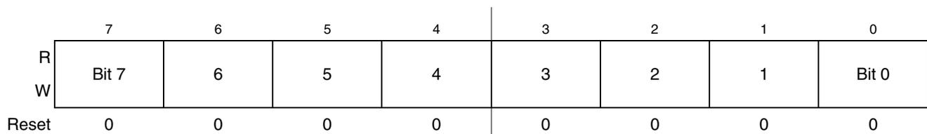
**Figure 10-12. Timer Channel Value Register Low (TPMxCnVL)**
