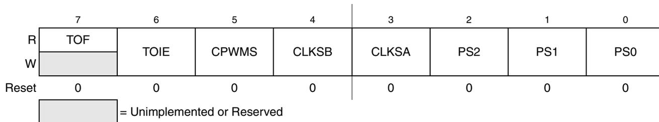
**Figure 10-5. Timer x Status and Control Register (TPMxSC)**
