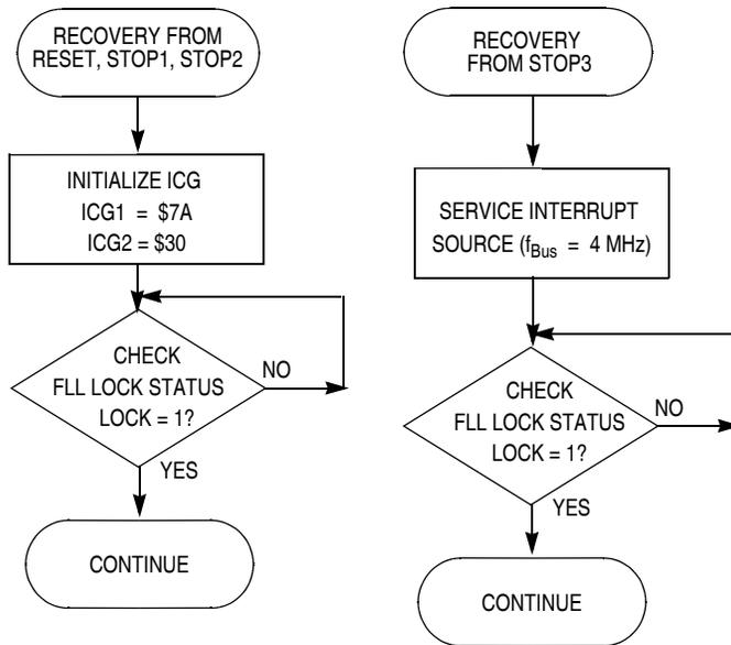
**Figure 7-9. ICG Initialization and Stop Recovery for Example #2**
