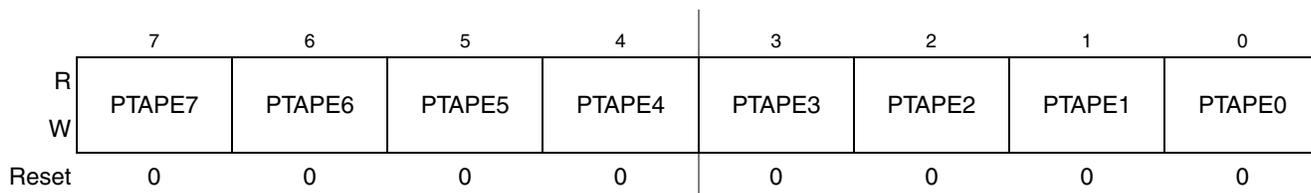
**Figure 6-10. Pullup Enable for Port A (PTAPE)**
