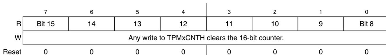
**Figure 10-6. Timer x Counter Register High (TPMxCNTH)**
