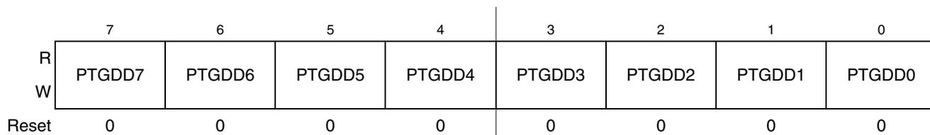
Figure 6-36. Data Direction for Port G (PTGDD)
