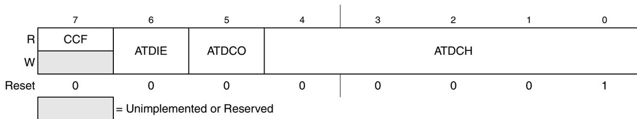
**Figure 14-6. ATD Status and Control Register (ATD1SC)**
