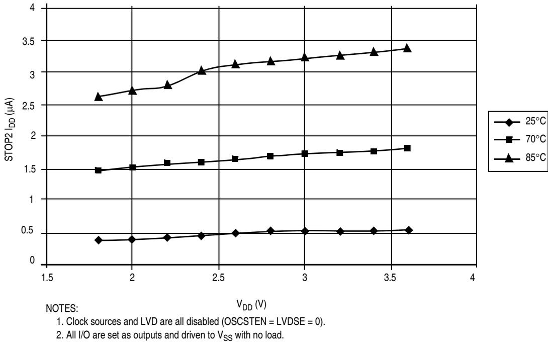
Figure A-8. Typical Stop 2 I<sub>DD</sub>
