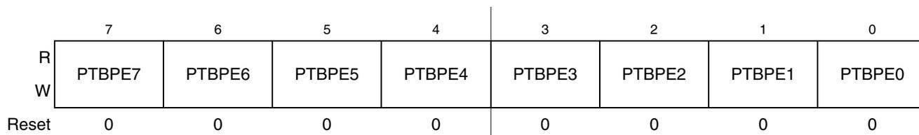
Figure 6-14. Pullup Enable for Port B (PTBPE)
