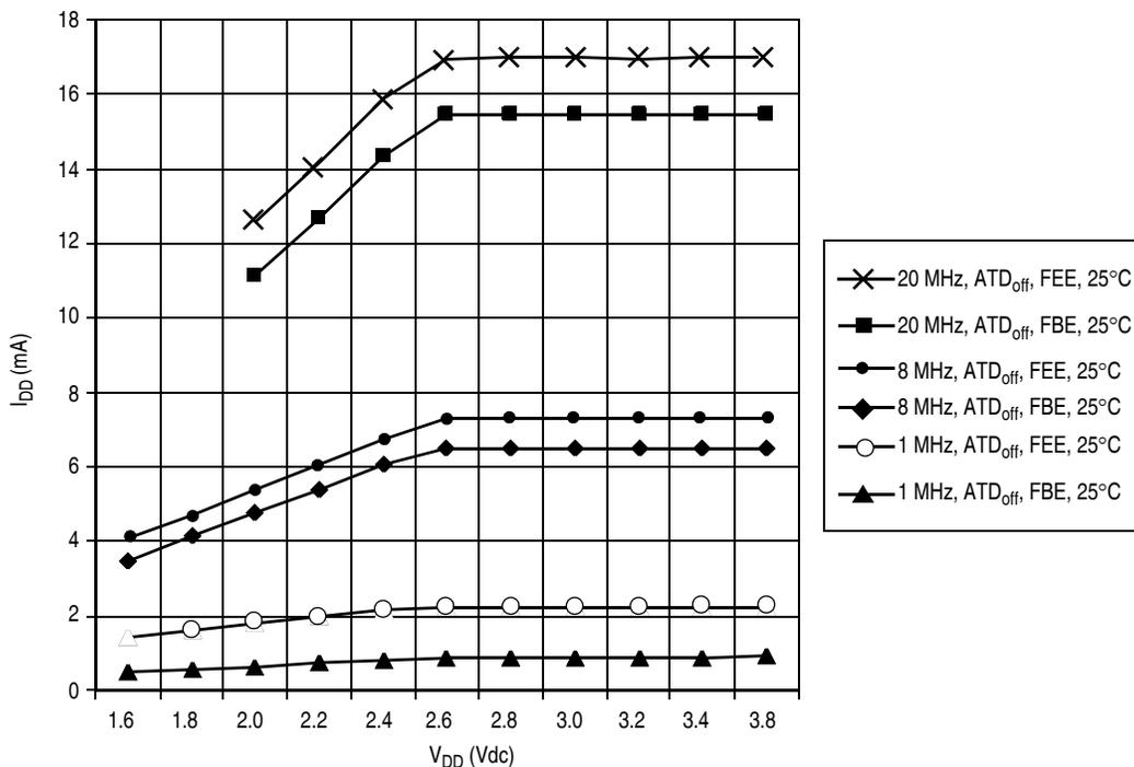
Figure A-6. Typical Run I<sub>DD</sub> for FBE and FEE Modes, I<sub>DD</sub> vs V<sub>DD</sub>
