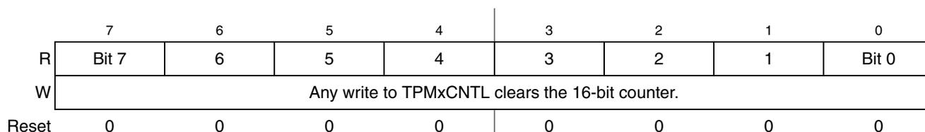
**Figure 10-7. Timer x Counter Register Low (TPMxCNTL)**
