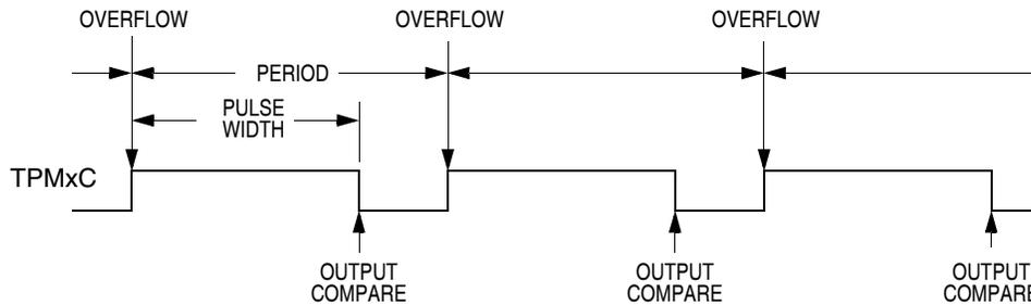
Figure 10-3. PWM Period and Pulse Width (ELSnA = 0)
