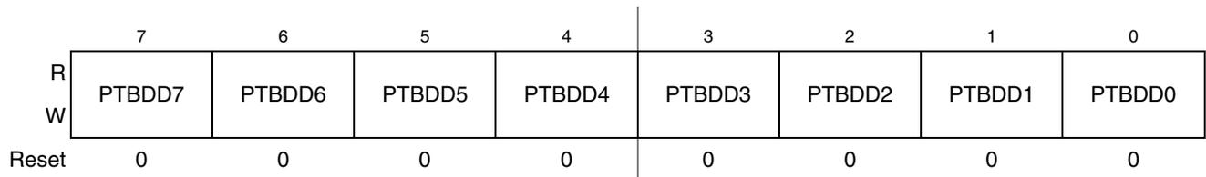
Figure 6-16. Data Direction for Port B (PTBDD)
