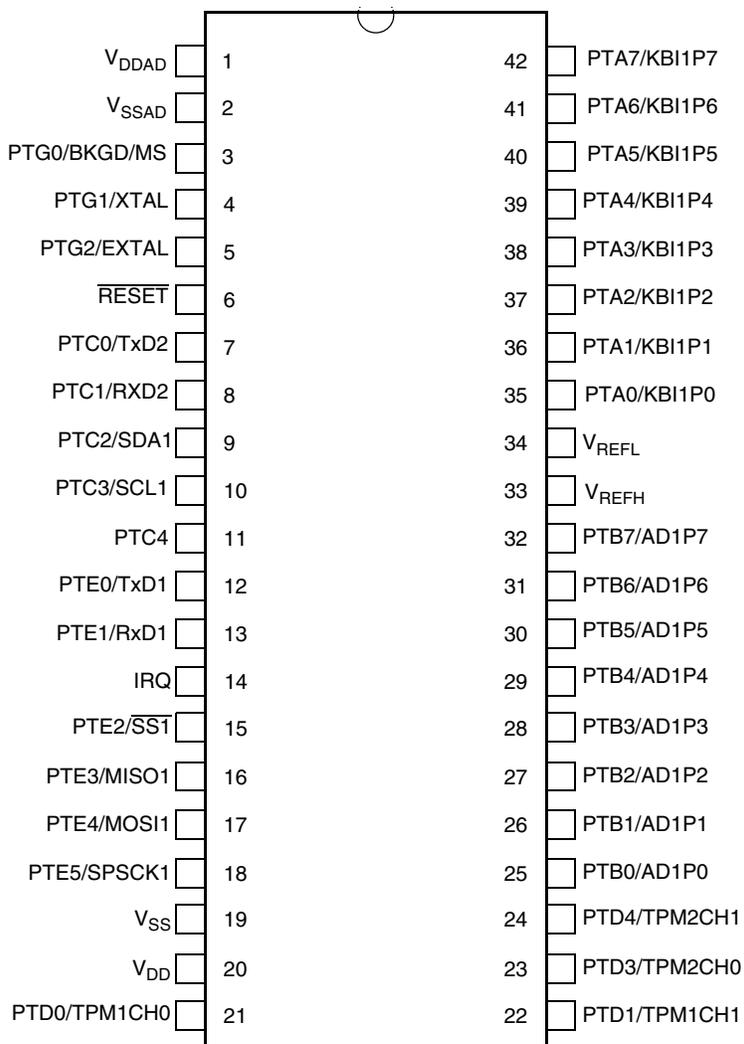
Figure 2-4. . MC9S08GTxxA in 42-Pin SDIP Package
