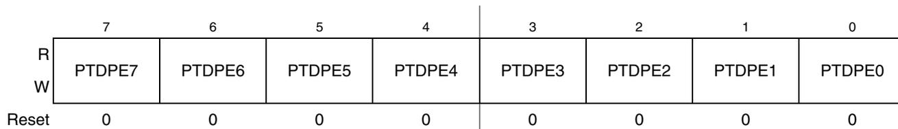
Figure 6-22. Pullup Enable for Port D (PTDPE)
