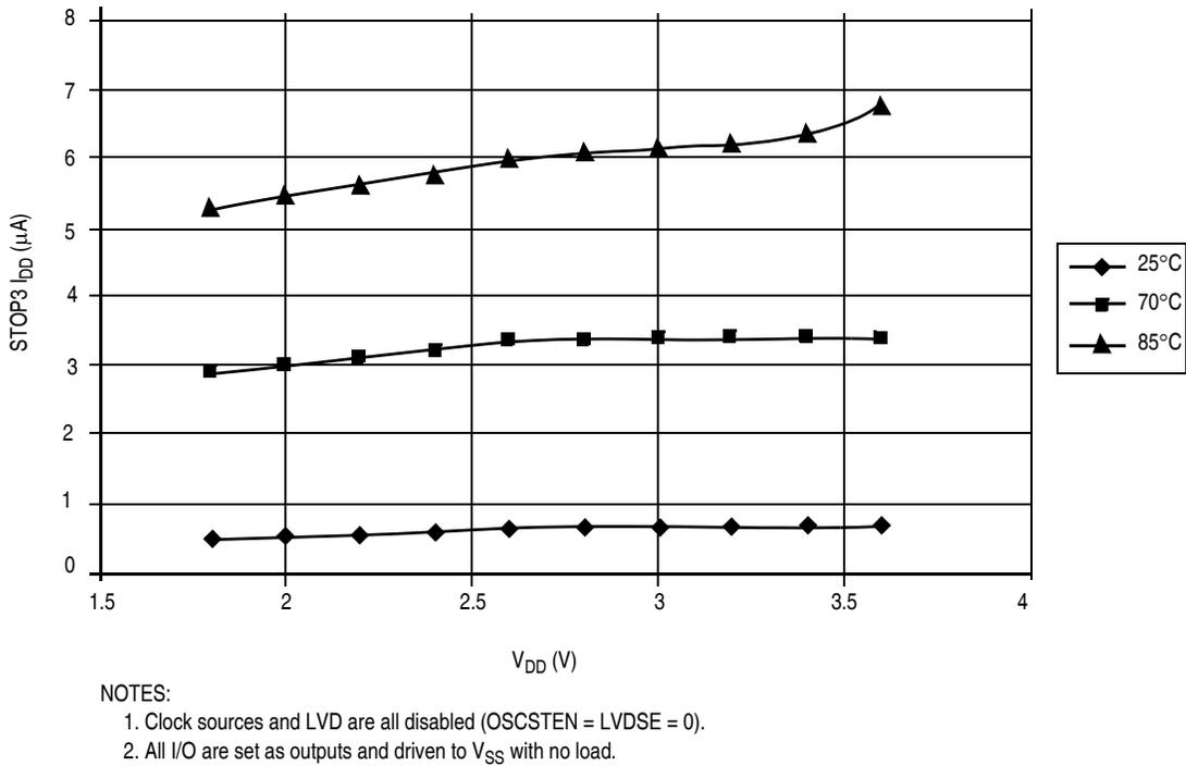
Figure A-9. Typical Stop3 I<sub>DD</sub>
