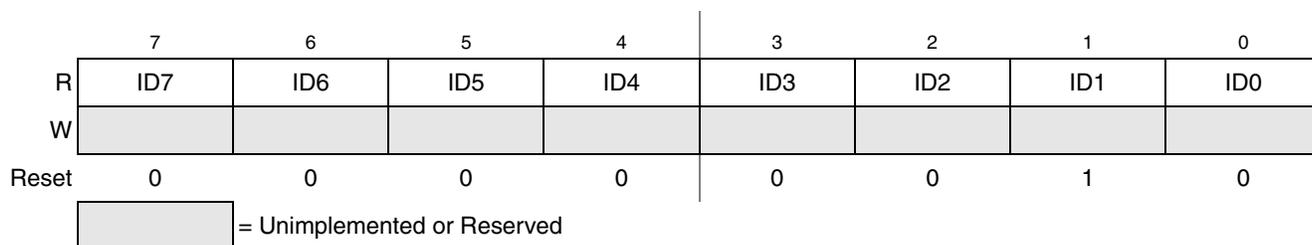
**Figure 5-7. System Device Identification Register Low (SDIDL)**
