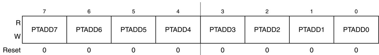
Figure 6-12. Data Direction for Port A (PTADD)
