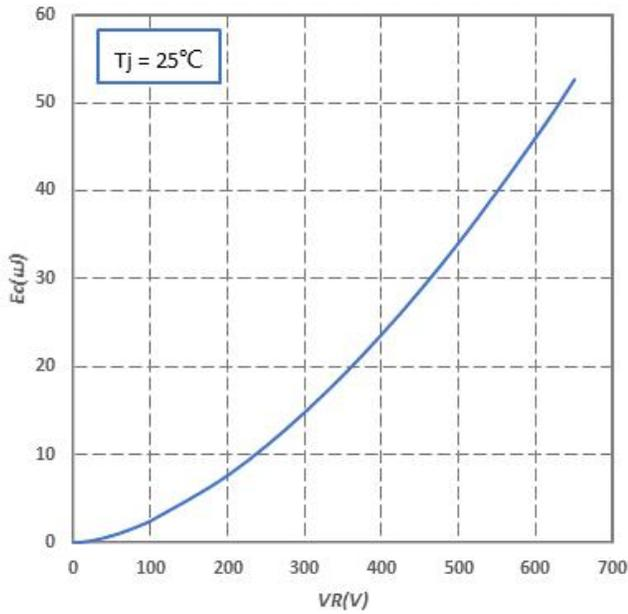
Fig.5-Capacitance Stored Energy
