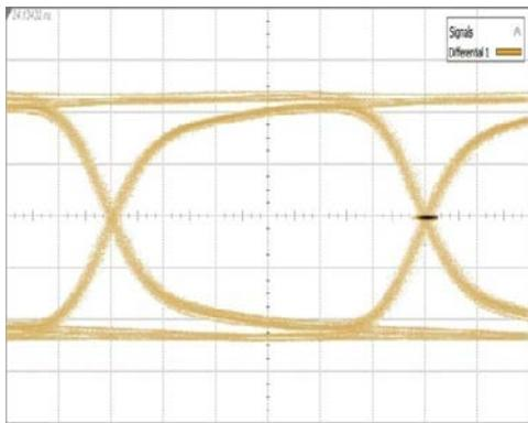
Figure 7. Output Eye Diagram at CPRI  $\times 12 = 6.144\text{ Gbps}$ ,
