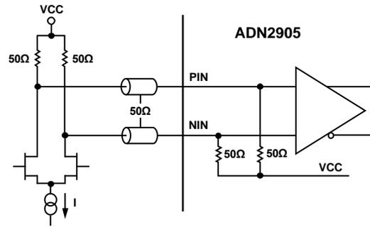
Figure 27. DC-Coupled Application, Bypass Input (Back Terminated Mode)
