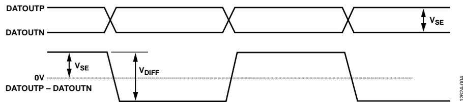
Figure 4. Single-Ended vs. Differential Output Amplitude Relationship
