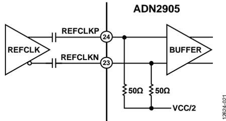
Figure 21. AC-Coupled, Differential REFCLKx Configuration
