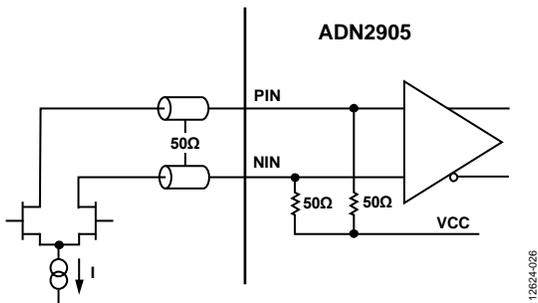
Figure 26. DC-Coupled Application, Bypass Input (Normal Mode)
