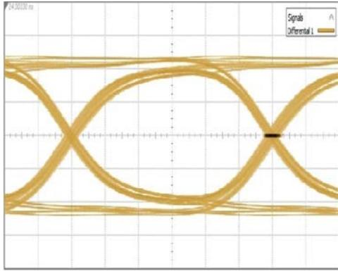
Figure 6. Output Eye Diagram at CPRI  $\times 16 = 9.8304\text{ Gbps}$ ,
