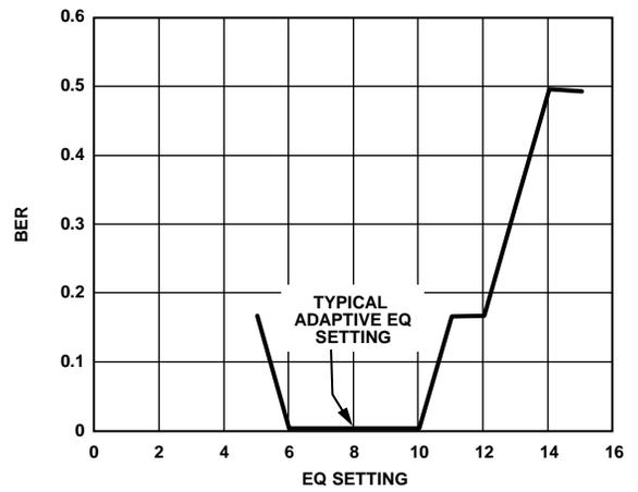
Figure 9. BER in Equalizer Mode vs. EQ Compensation at CPRI  $\times 16 = 9.8304\text{ Gbps}$  (with a Signal of 400 mV p-p Differential, on 15 inch FR4 Traces, with Variant EQ Compensation, Including Adaptive EQ)
