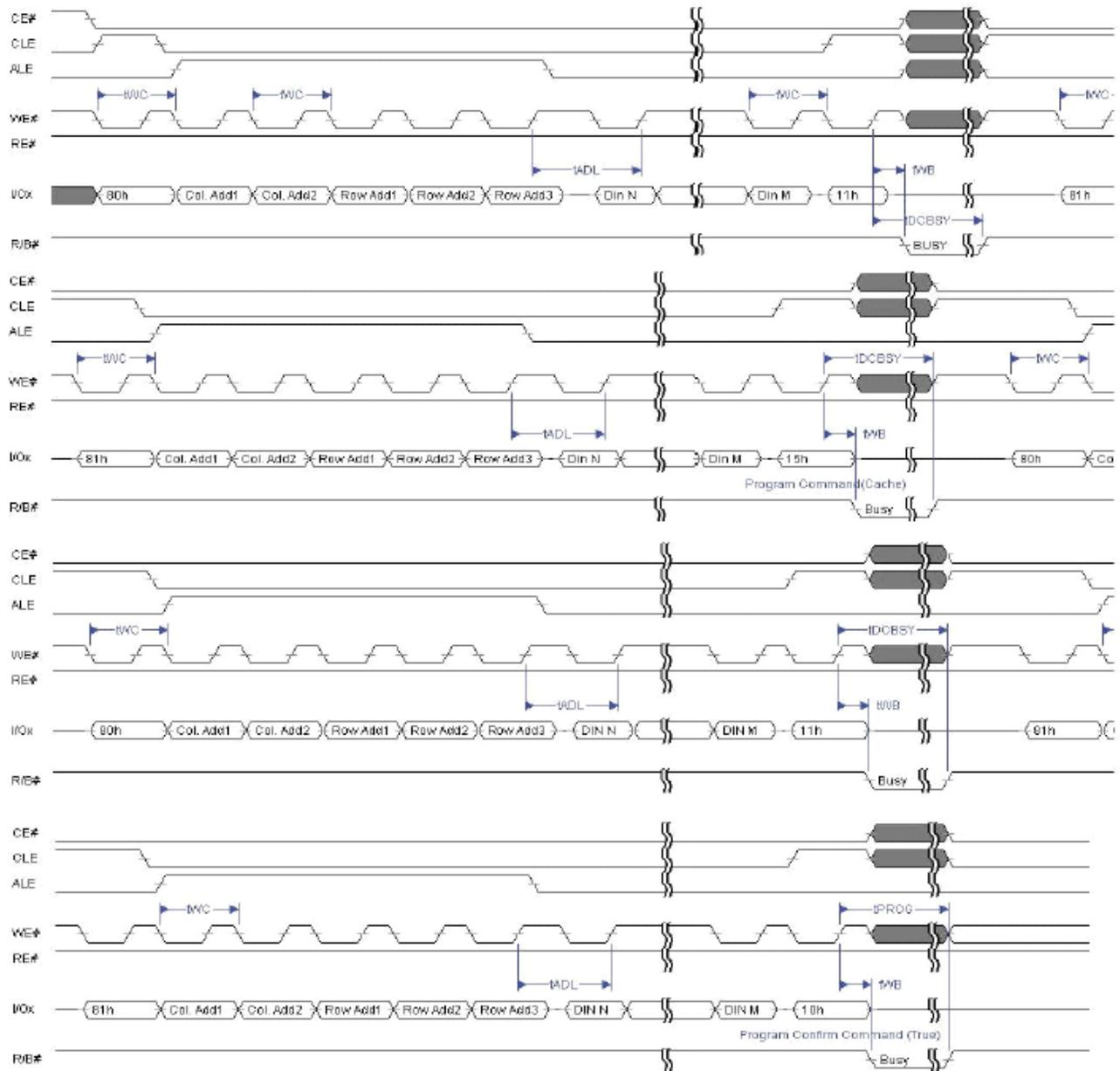
**Figure 6.20 Two-Plane Cache Program Operation**
