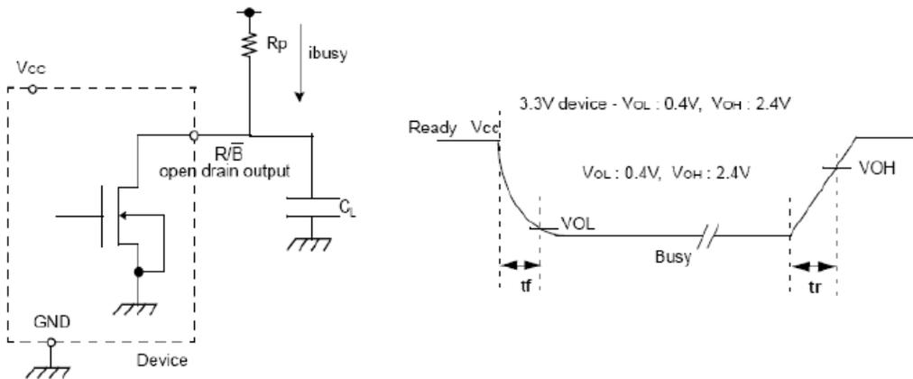
$R_p$  vs  $t_{RHOH}$  vs  $C_L$
