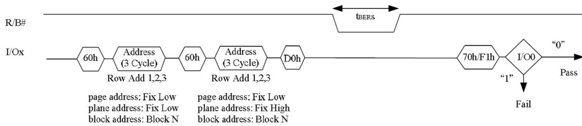
Figure 8.18 Two-Plane Block Erase
