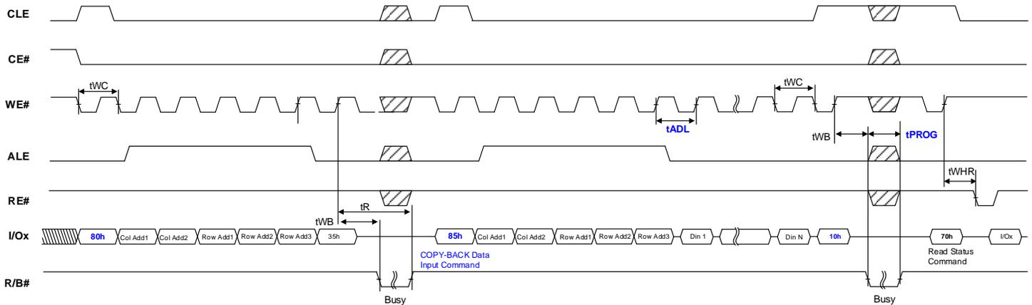
**Figure 6.12 Copy-Back Operation with Random Data Input**
