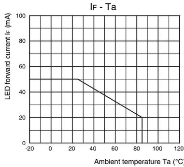
Continuous load current vs. Ambient temperature
