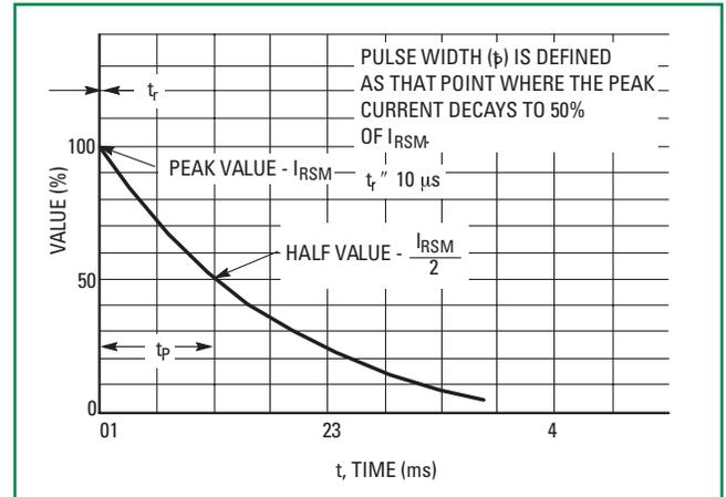
**Figure 3. 8 X 20  $\mu\text{s}$  Pulse Waveform**
