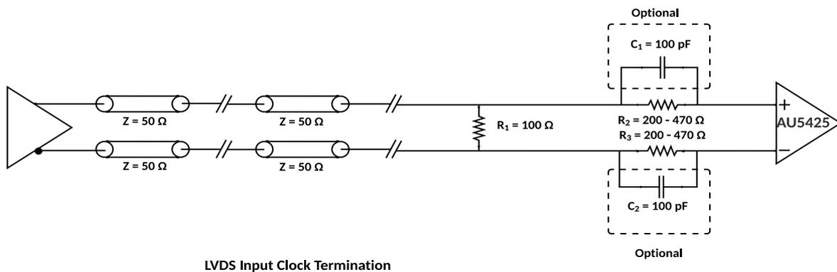
Figure 31 LVDS termination with hot swap protection
