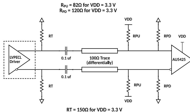
Figure 20 Termination scheme for AC coupled LVPECL, Thevenin Equivalent
