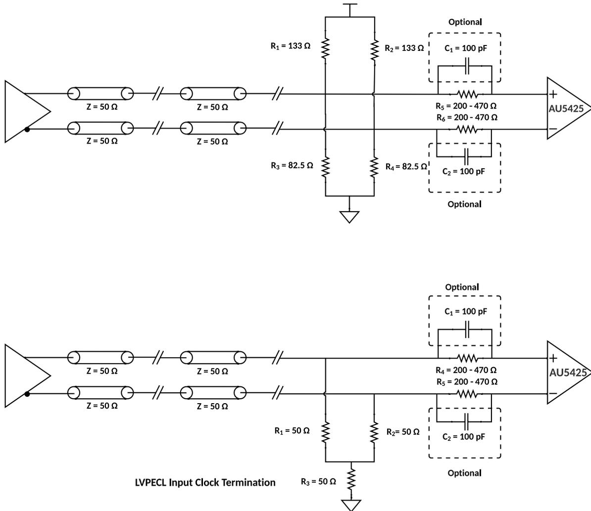
Figure 30 LVPECL termination with hot swap protection
