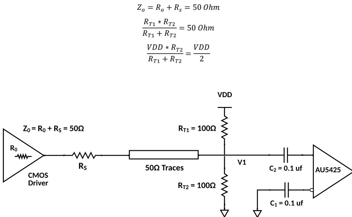
Figure 6 AC coupling LVCMOS clock to AU5425
