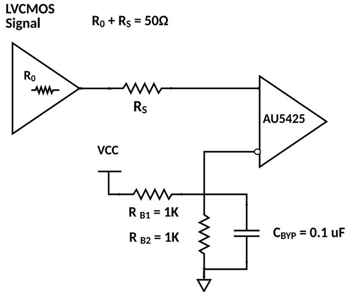
Figure 11: Direct coupling of LVCMOS clock to AU5425
