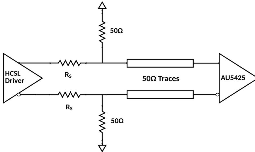
Figure 15 Termination scheme for DC coupled HCSL
