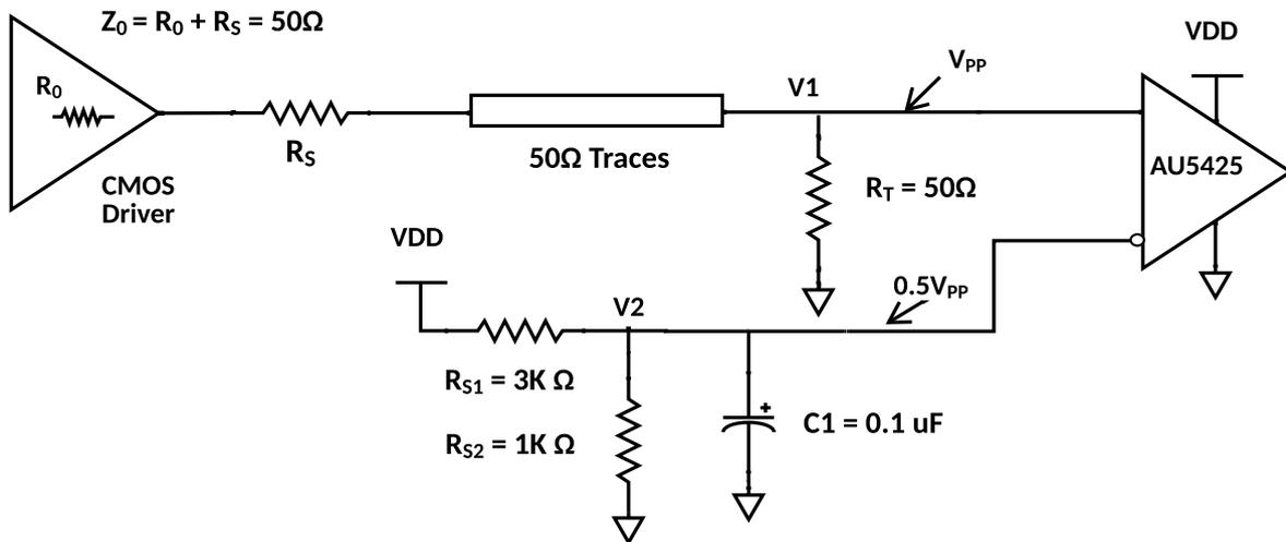
Figure 9 DC coupled LVCMOS input clock configuration – configuration 2
