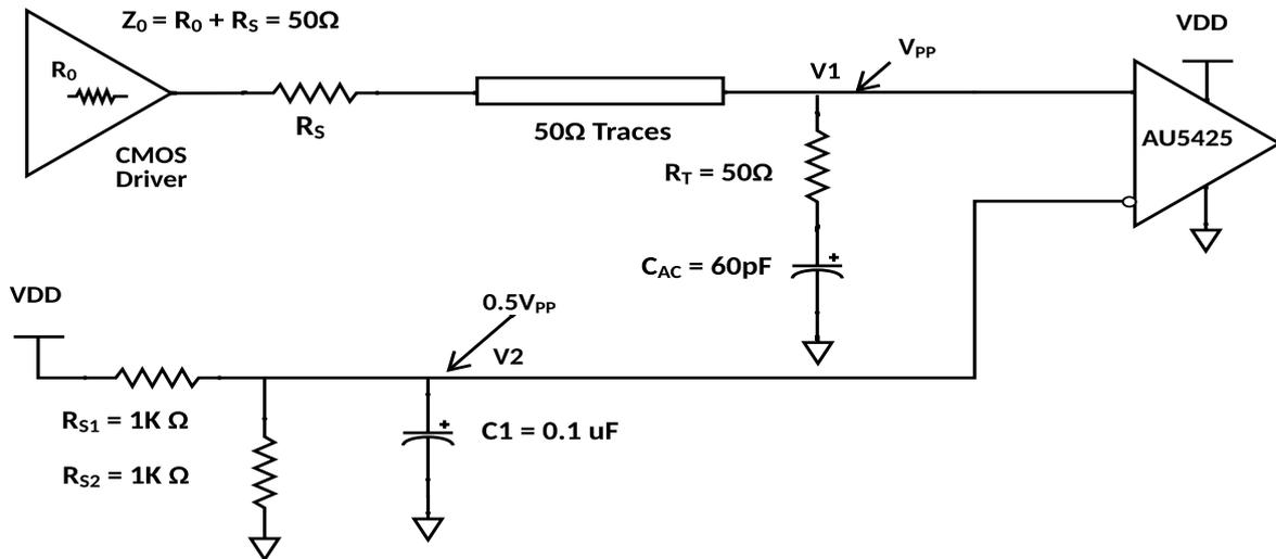
Figure 10 DC coupled LVCMOS input clock with series RC termination – configuration 3
