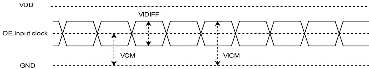
Figure 26 Parameters related to differential input level
