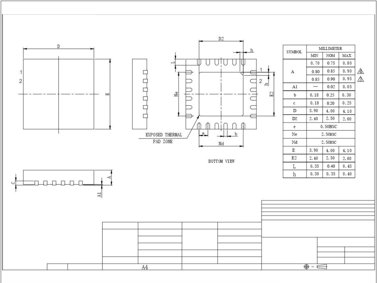
Figure 36 AU5425 24 Pin QFN Package Information
