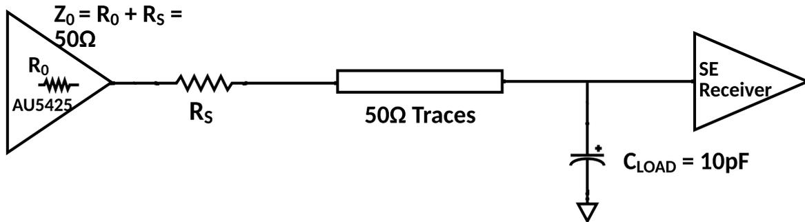
Figure 25 Typical application load
