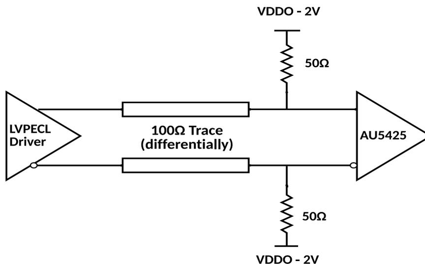
Figure 16 Termination scheme for DC coupled LVPECL
