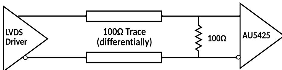
Figure 14 Termination scheme for DC coupled LVDS
