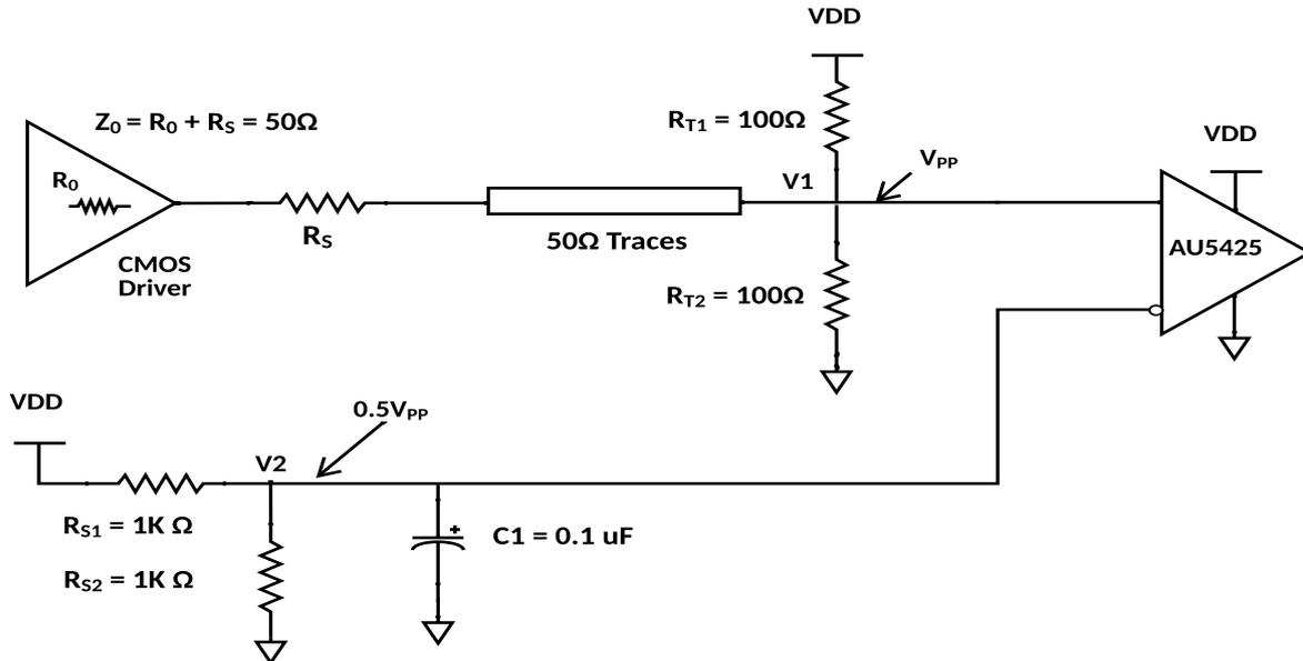
Figure 8 DC coupling of LVCMOS clock to AU5425 – configuration 1
