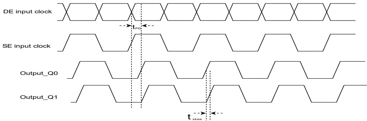
Figure 27 Parameter definitions of propagation delay and skew
