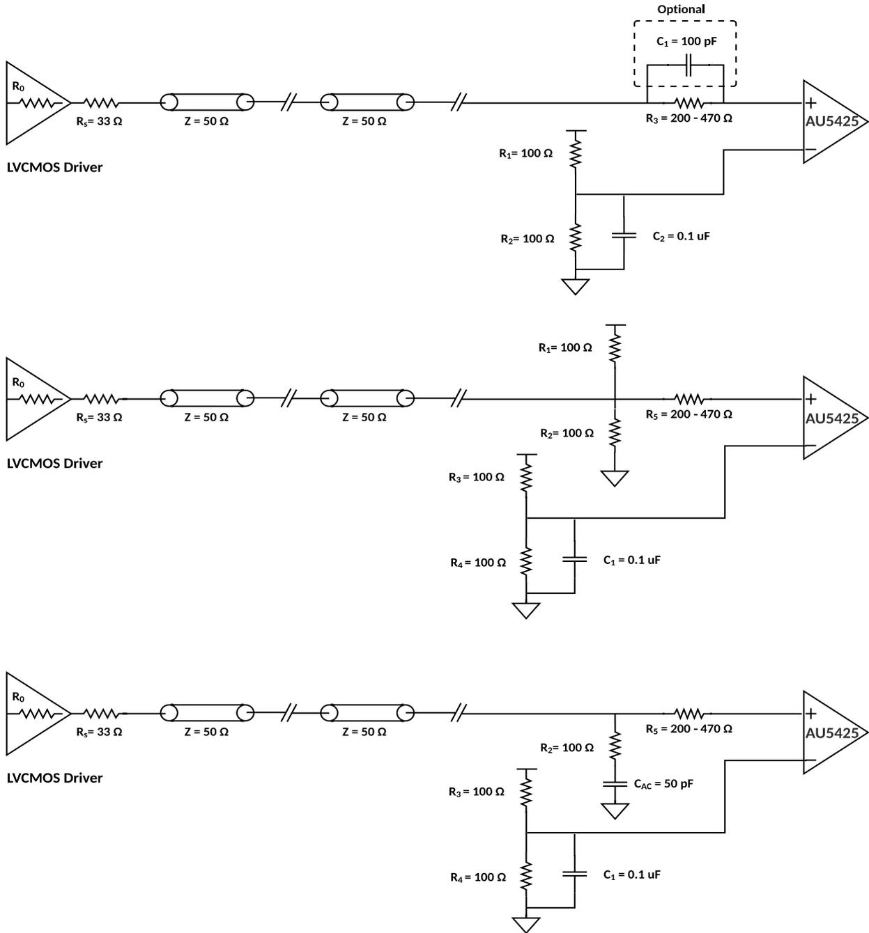
Figure 33 LVCMOS Input Clock Termination with Hot Swap Protection
