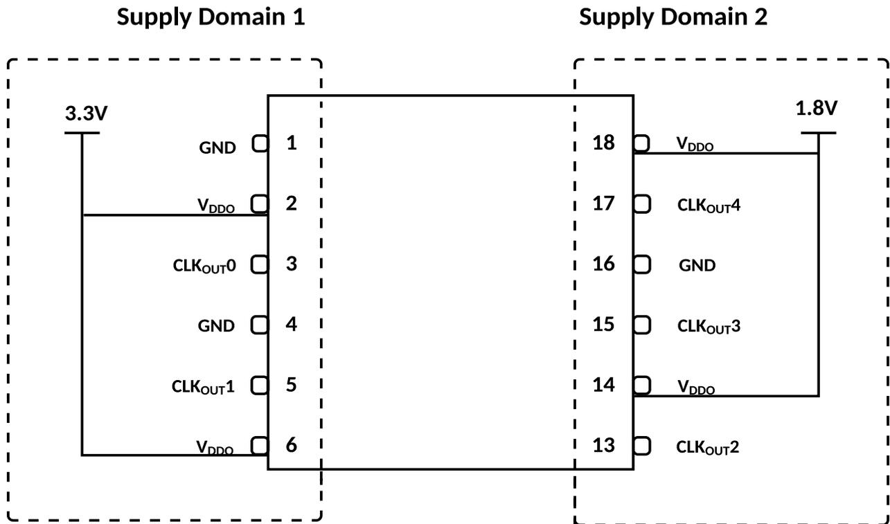
Figure 35 Example of multi supply operation of AU5425
