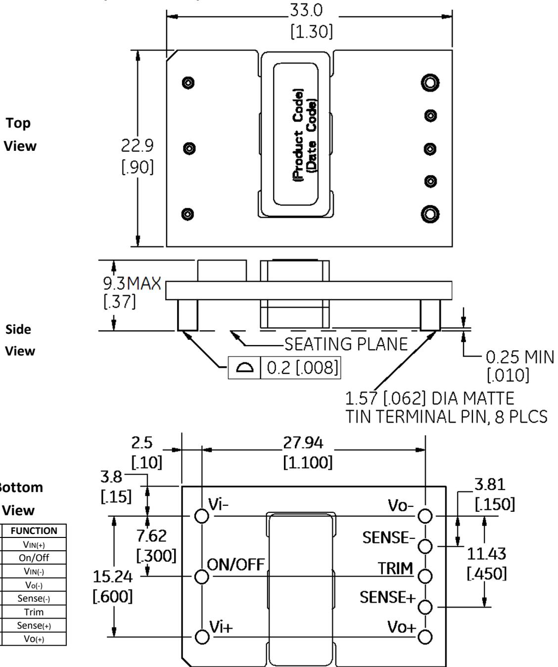
**KHHD006A0A Hammerhead™ Series; DC-DC Converter Power Modules**
