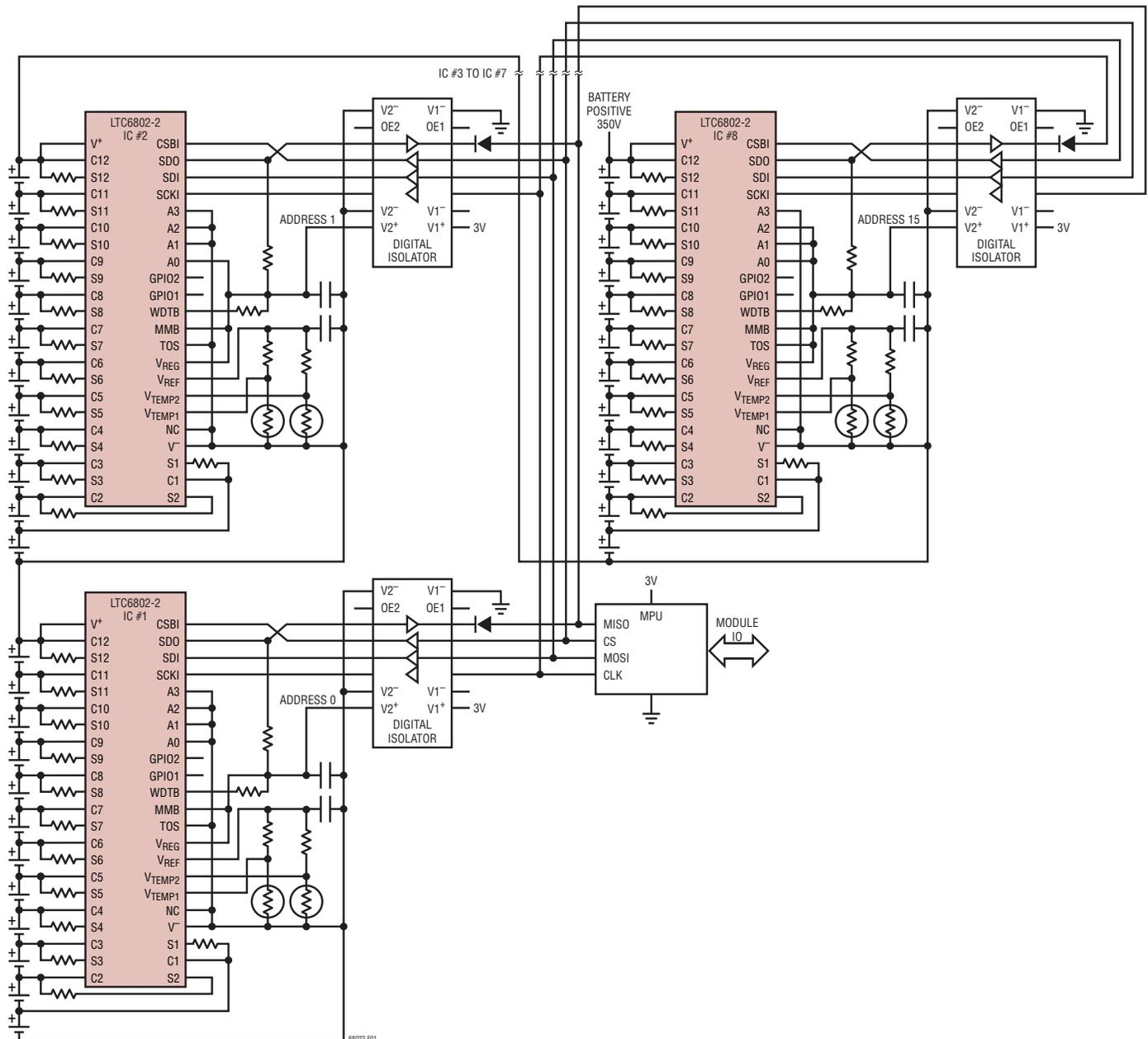
**Figure 1. 96-Cell Battery Stack, Isolated Interface.** In this Diagram the Battery Negative is Isolated from Module Ground. Opto-Couplers or Digital Isolators Allow Each IC to be Addressed Individually. This is a Simplified Schematic Showing the Basic Multi-IC Architecture
