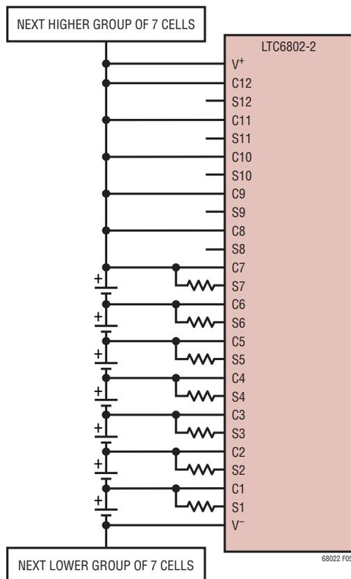
Figure 5. Monitoring 7 Cells with the LTC6802-2
