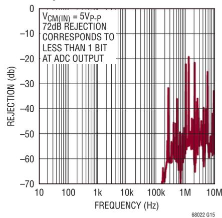
**ADC Normal Mode Rejection vs Frequency**
