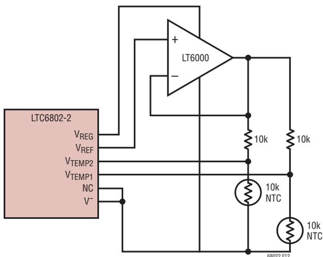
Figure 12. Buffering  $V_{REF}$  for Higher Current Sensors
