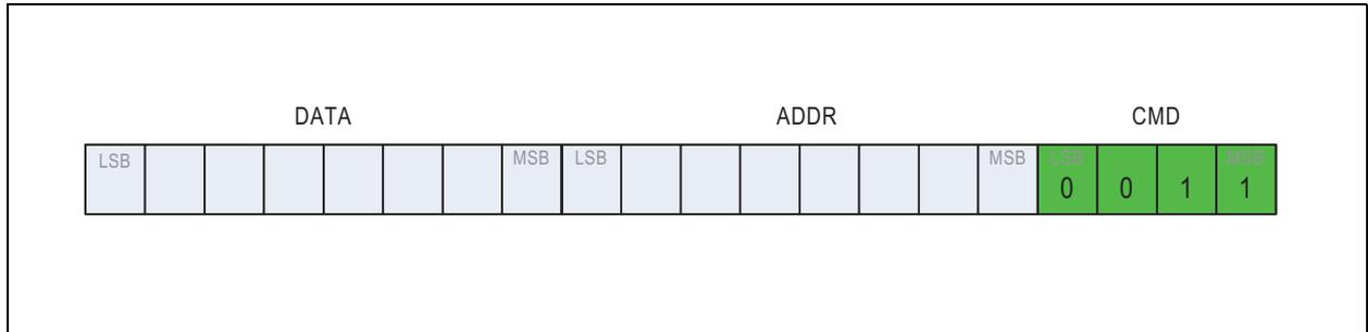
The command consists of one frame received by the AS5263 (slave communication mode). The data byte will be written to the address. The access is performed with CMD field set to 0xC.
