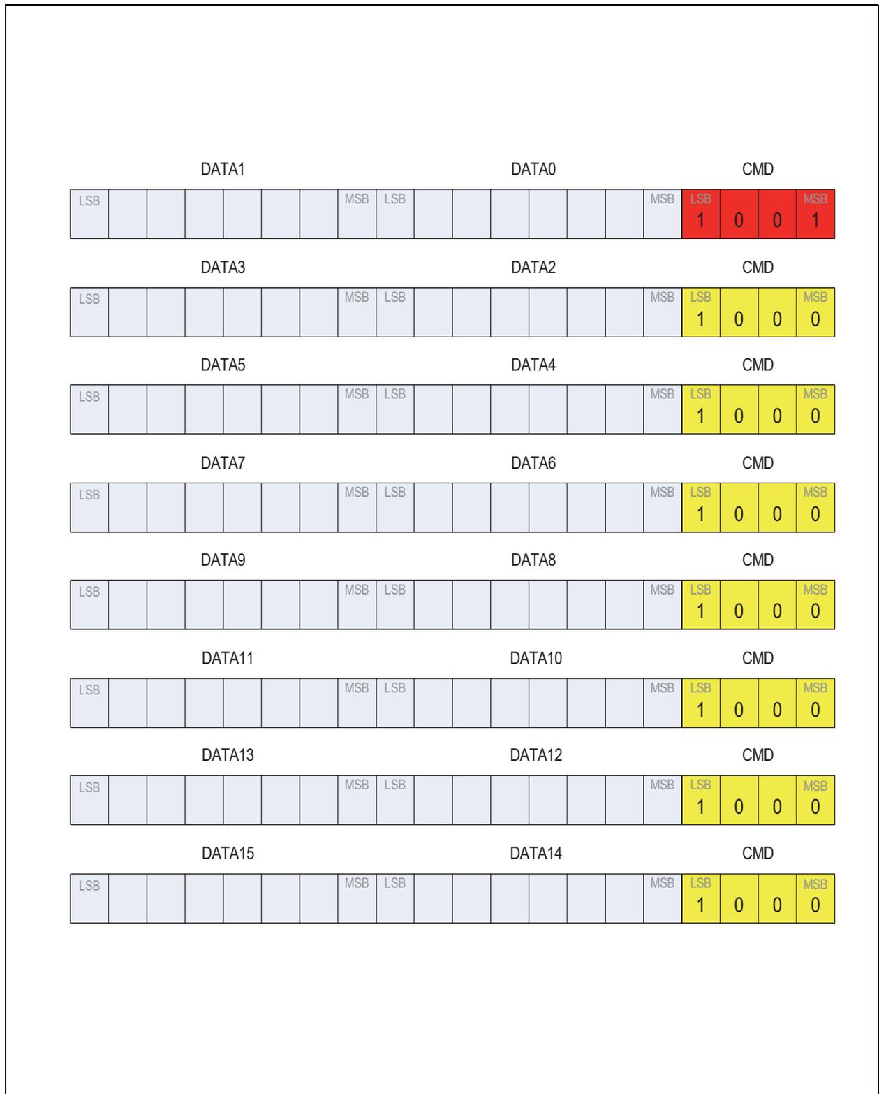
The command contains 8 frames. With this command, the AS5263 receives only frames. This command will transfer the data in the special function registers (SFRs) of the device. The data is not permanent programmed using this command.
