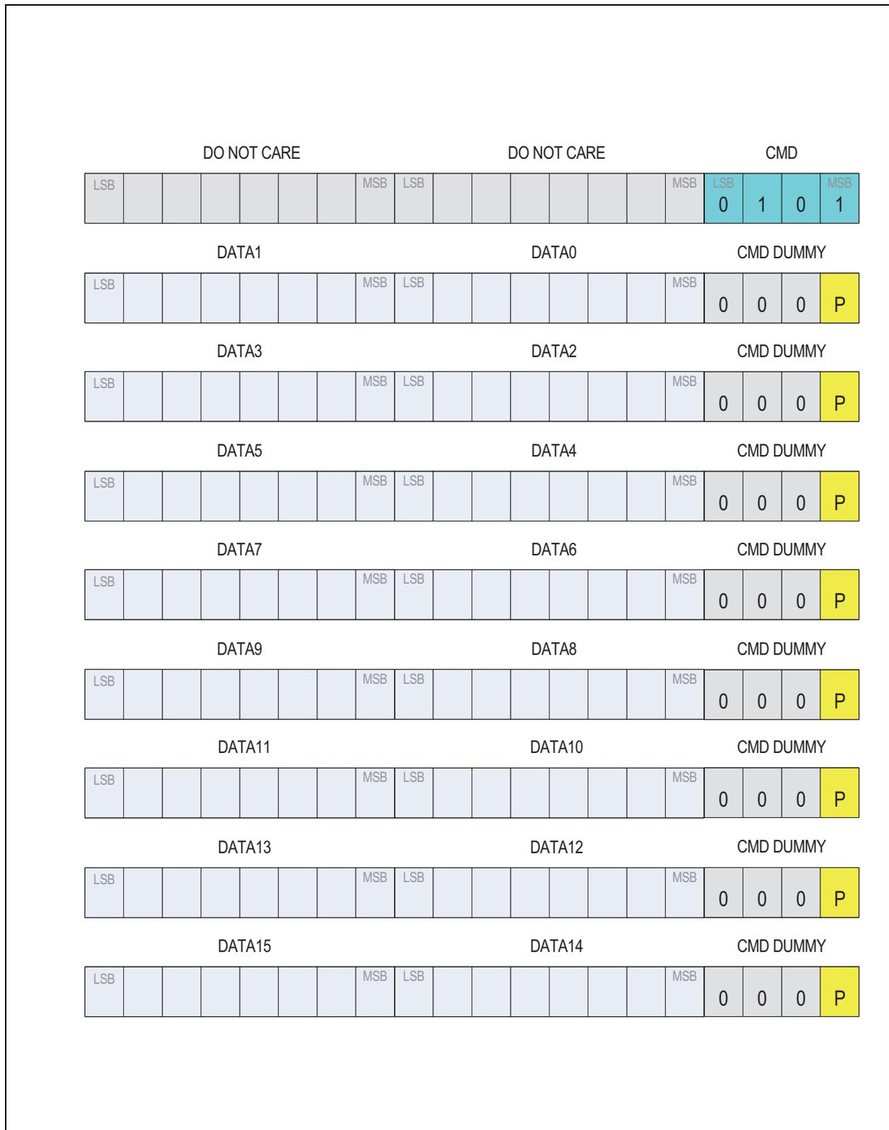
The command is composed by a first frame transmitted to the AS5263. The device is in slave communication mode. The device remains for the time  $T_{SWITCH}$  in IDLE mode before changing into the master communication mode. The AS5263 starts to send 8 frames. This command will read the SFRs. The numbering of the data bytes correlates with the address of the related SFR.
