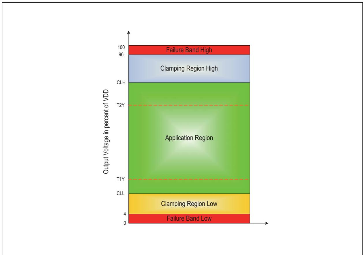
Figure 17 gives an overview of the different ranges. The failure bands are used to indicate a wrong operation of the AS5263. This can be caused due to a broken supply line. By using the specified load resistors, the output level will remain in these bands during a fail. It is recommended to set the clamping level **CLL** above the lower failure band and the clamping level **CLH** below the higher failure band.
