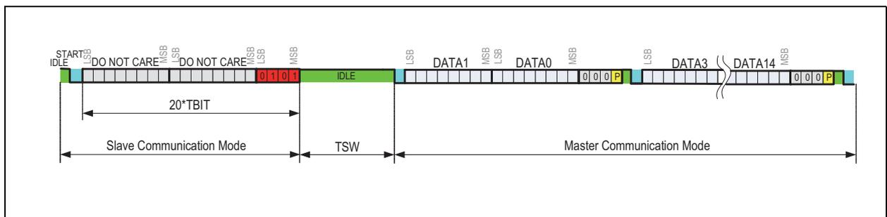
In case of READ or READ128 command (see Figure 32) the idle phase between the command and the answer is 10 TBIT (TSW).
