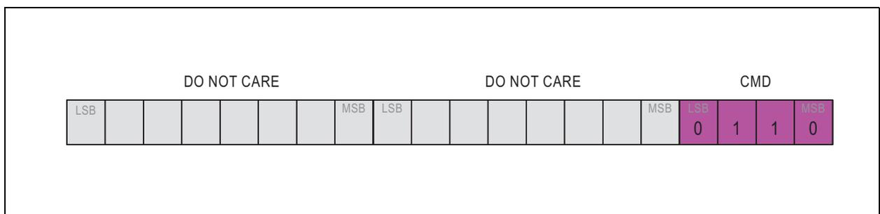
The command consists of one frame received by the AS5263 (slave communication mode) and transfers the data from the SFRs into the OTP fuse cells. The OTP fuses are not permanent programmed using this command.
