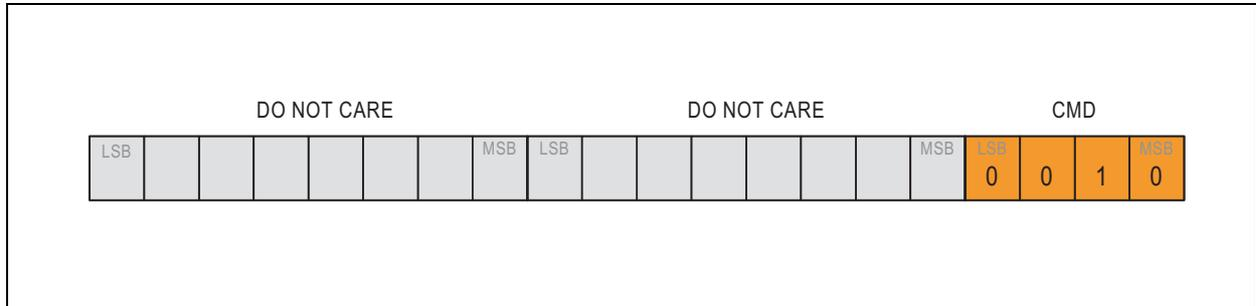
The command consists of one frame received by the AS5263 (slave communication mode) and it is giving the trigger to permanent program the non volatile fuse elements.
