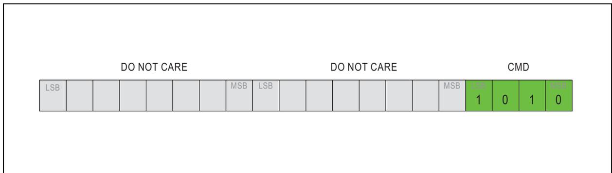
The command consists of one frame received by the AS5263 (slave communication mode). The OTP cell fuse content will be downloaded into the SFRs.
