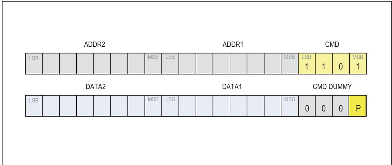
The command is composed by a first frame sent to the AS5263. The device is in slave communication mode. The device remains for the time  $T_{SWITCH}$  in IDLE mode before changing into the master communication mode. The AS5263 starts to send the second frame transmitted by the AS5263.
