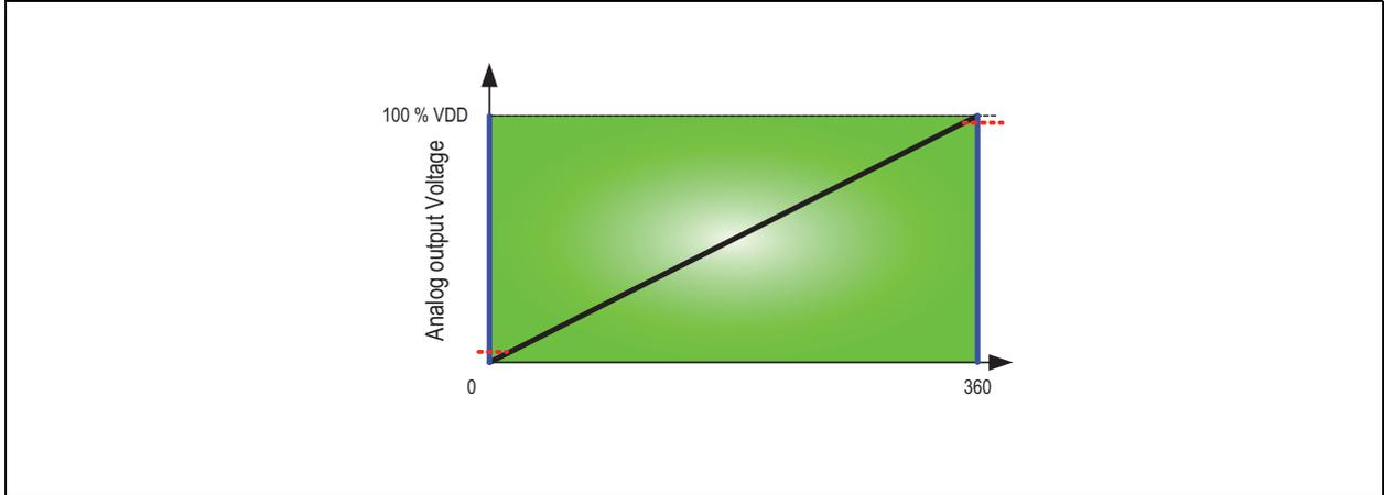
For simplification, [Figure 14](#) describes a linear output voltage from rail to rail (0V to VDD) over the complete rotation range. In practice, this is not feasible due to saturation effects of the output stage transistors. The actual curve will be rounded towards the supply rails (as indicated [Figure 14](#)).
