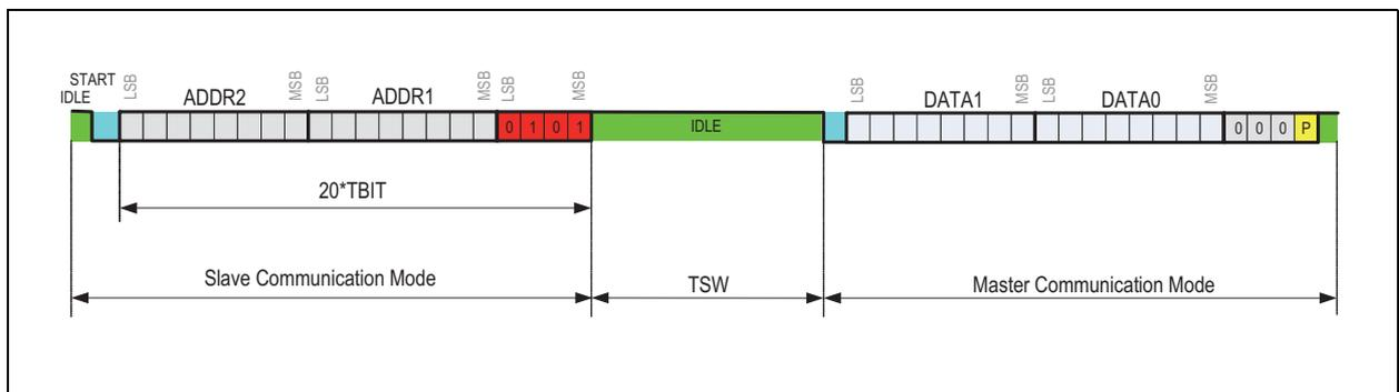
In case of a WRITE command, the device stays in slave communication mode and will not switch to master communication mode.
