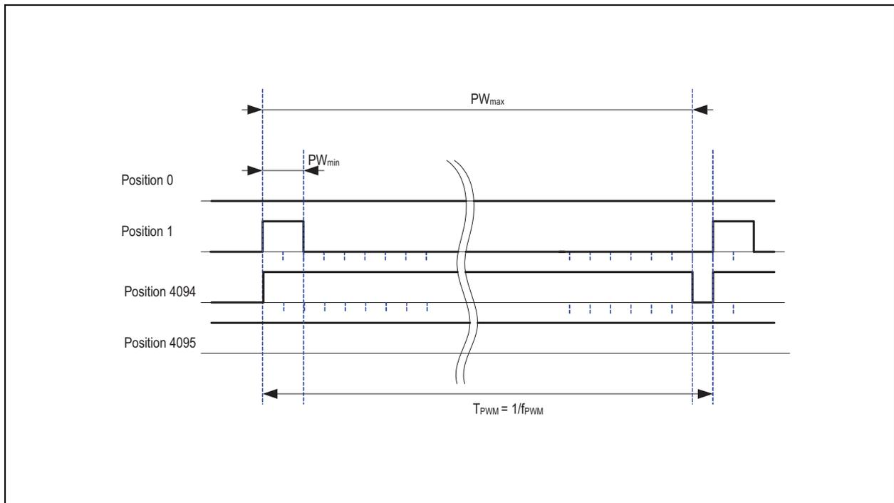
The PWM frequency can be programmed by the OTP bits **PWM\_frequency (1:0)**. Therefore, four different frequencies are possible.
