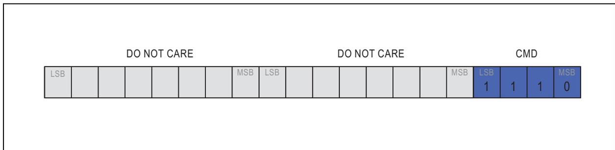
The command consists of one frame received by the AS5263 (slave communication mode). This command stops the communication receiving mode, releases the reset of the DSP of the AS5263 device and starts to work in functional mode with the values of the SFR currently written.
