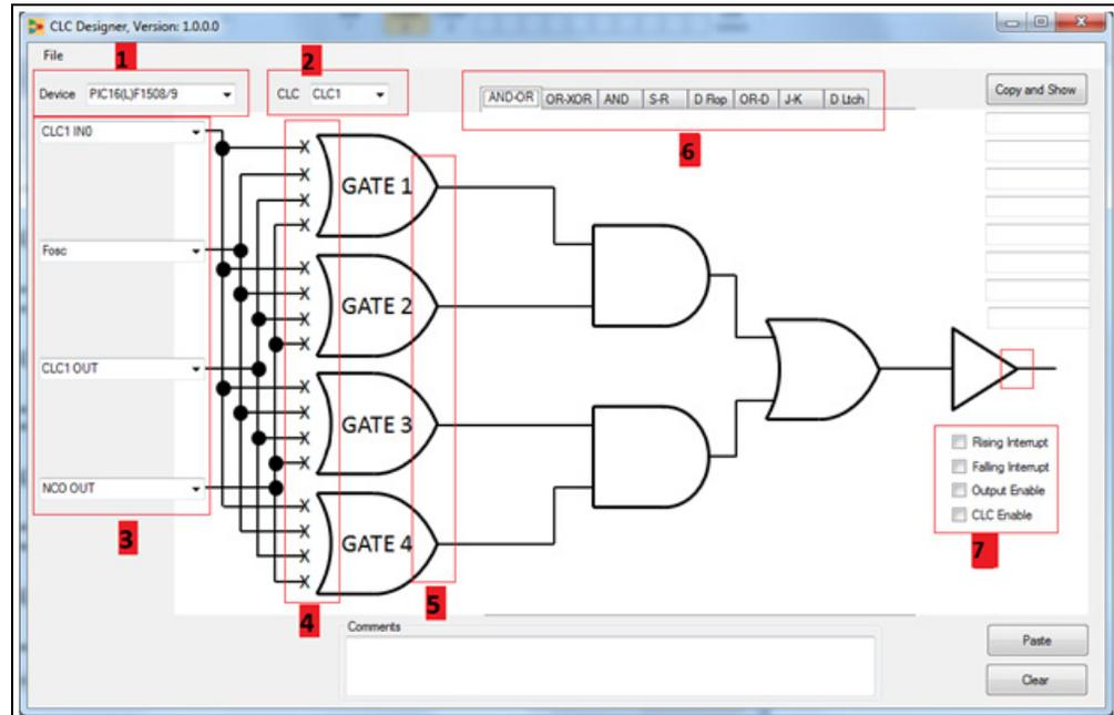
The CLC Configuration Tool provides a friendly alternative to manually configuring the 8 CLC registers for each module in software. Table 1-1 correlates each block in the above figure with its matching register in the device's data sheet.
