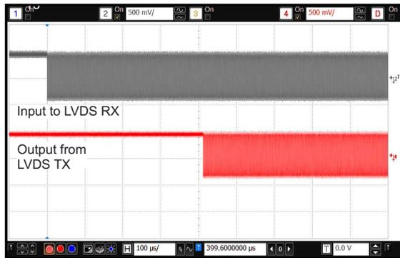
Figure 15. Distortion Correction Scheme Calibration Time ( $t_{CALIB}$ )
