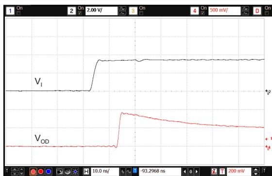
Figure 17. Disable to Enable Time ( $t_{PZH}$ )
