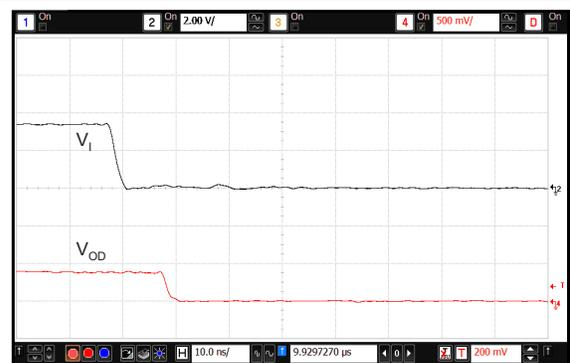
Figure 18. Disable Time ( $t_{PLZ}$ ,  $t_{PHZ}$ )
