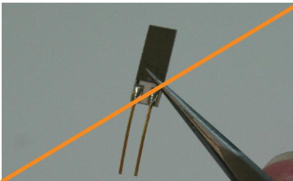
Picture 5: Sensor picked on the active area with metal tweezers
