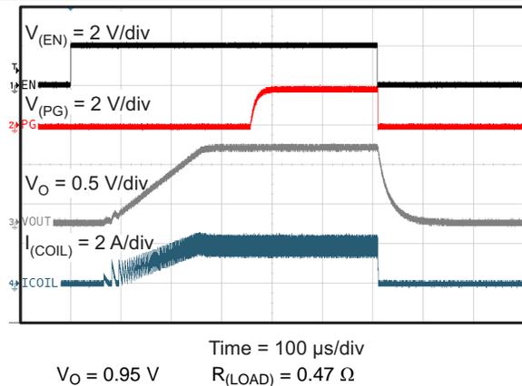
Figure 15. TPS62134A Startup and Shutdown
