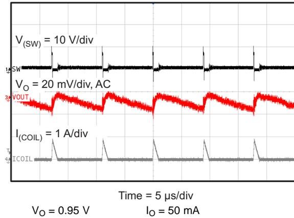
Figure 13. TPS62134A Output Ripple
