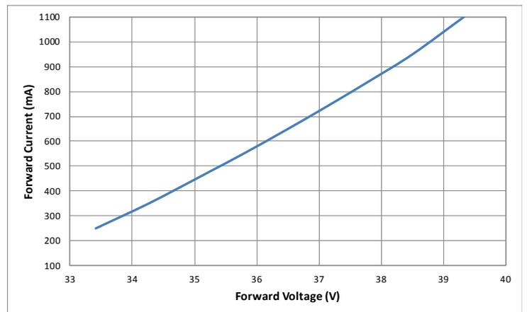
**CXM-11 & CXM-14 Optical & Electrical Characteristics**
