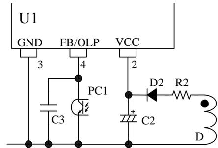
Figure 9-12 FB/OLP pin peripheral circuit
