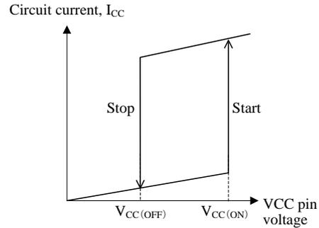
Figure 9-2 Relationship between VCC pin voltage and  $I_{CC}$
