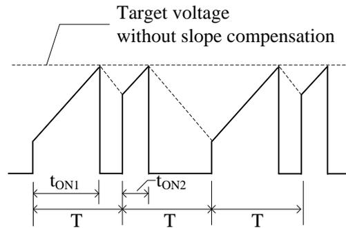
Figure 9-7 Drain current,  $I_D$ , waveform in subharmonic oscillation
