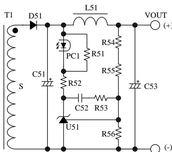
Figure 10-3 Peripheral circuit of secondary side shunt regulator ( $U1$ )
