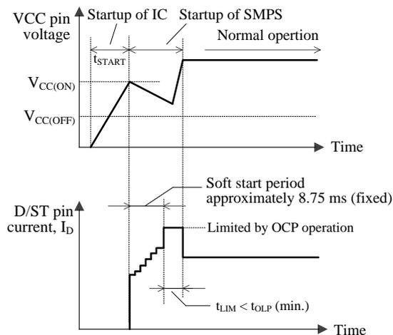
Figure 9-4  $V_{CC}$  and  $I_D$  behavior during startup
