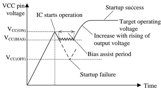
Figure 9-3 VCC pin voltage during startup period
