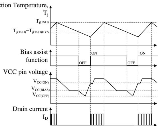
Figure 9-15 TSD operational waveforms
