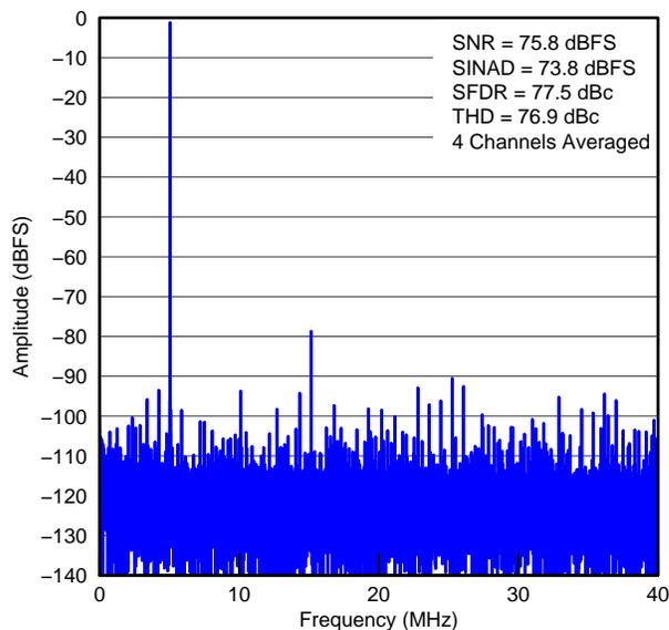
**Figure 31. FFT FOR 5-MHz INPUT SIGNAL**
