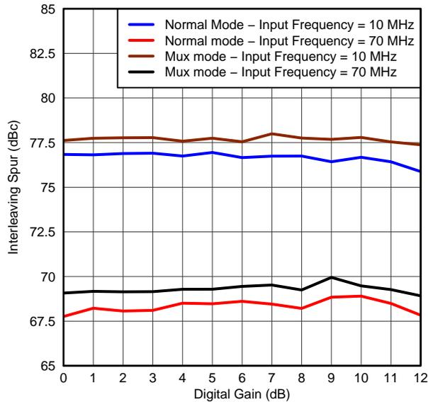
**Figure 49. INTERLEAVING SPUR ( $f_s / 2 - f_{IN}$ ) vs DIGITAL GAIN**
