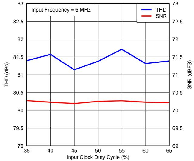
**Figure 19. PERFORMANCE vs INPUT CLOCK DUTY CYCLE**
