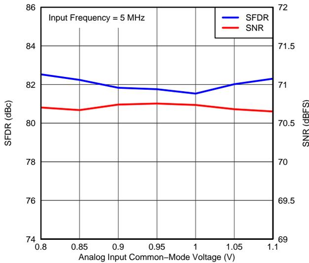
**Figure 20. PERFORMANCE vs INPUT COMMON-MODE VOLTAGE**
