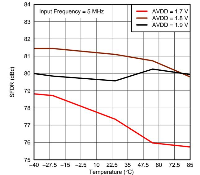
**Figure 52. SPURIOUS-FREE DYNAMIC RANGE vs AVDD AND TEMPERATURE**
