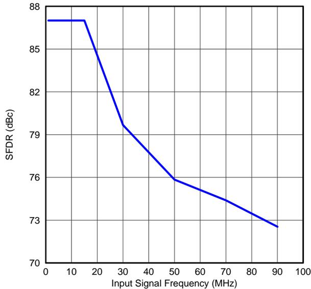
Figure 45. SPURIOUS-FREE DYNAMIC RANGE vs INPUT SIGNAL FREQUENCY
