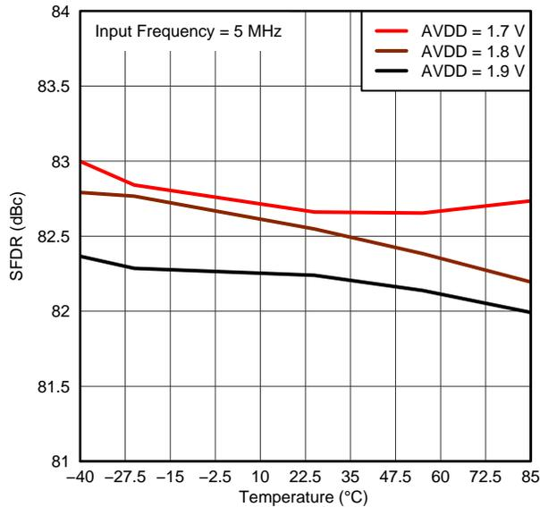
Figure 22. SPURIOUS-FREE DYNAMIC RANGE vs AVDD AND TEMPERATURE
