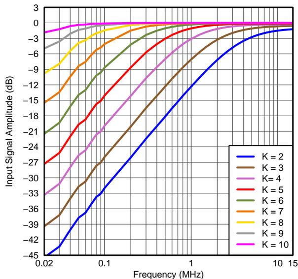
**Figure 32. DIGITAL HIGH-PASS FILTER RESPONSE** <sup>G027</sup>
