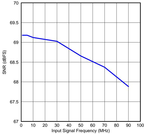
**Figure 61. SIGNAL-TO-NOISE RATIO vs INPUT SIGNAL FREQUENCY**
