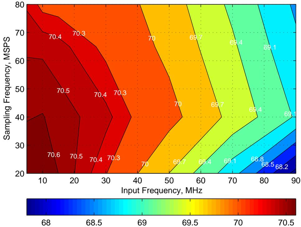
Figure 39. SIGNAL-TO-NOISE RATIO vs INPUT AND SAMPLING FREQUENCIES
