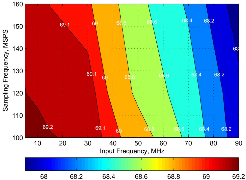
Figure 71. SIGNAL-TO-NOISE RATIO vs INPUT AND SAMPLING FREQUENCIES
