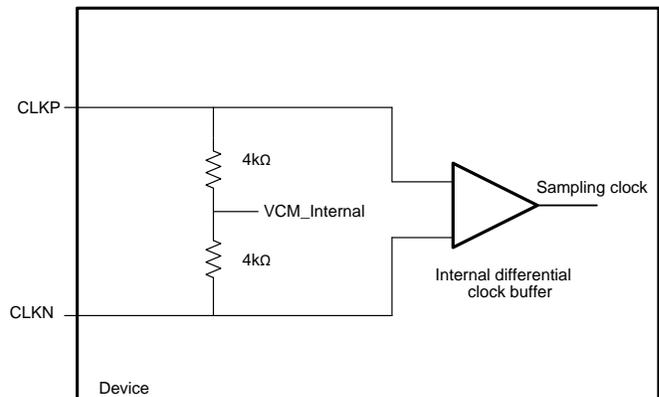
**Figure 90. Input Clock Equivalent Circuit: Differential Mode**
