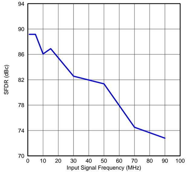
**Figure 62. SPURIOUS-FREE DYNAMIC RANGE vs INPUT SIGNAL FREQUENCY**
