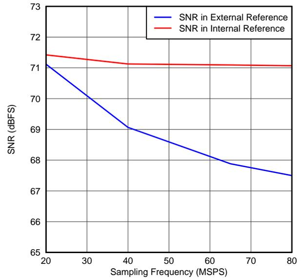
Figure 93. SNR in Internal and External Reference Mode
