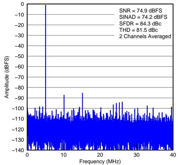
**Figure 29. FFT FOR 5-MHz INPUT SIGNAL (Sample Rate = 80 MSPS by Averaging Two Channels)<sup>(1)</sup>**
