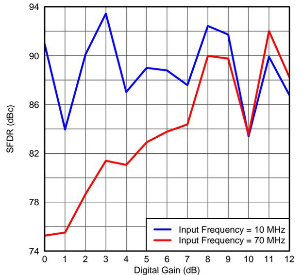
Figure 48. SPURIOUS-FREE DYNAMIC RANGE vs DIGITAL GAIN
