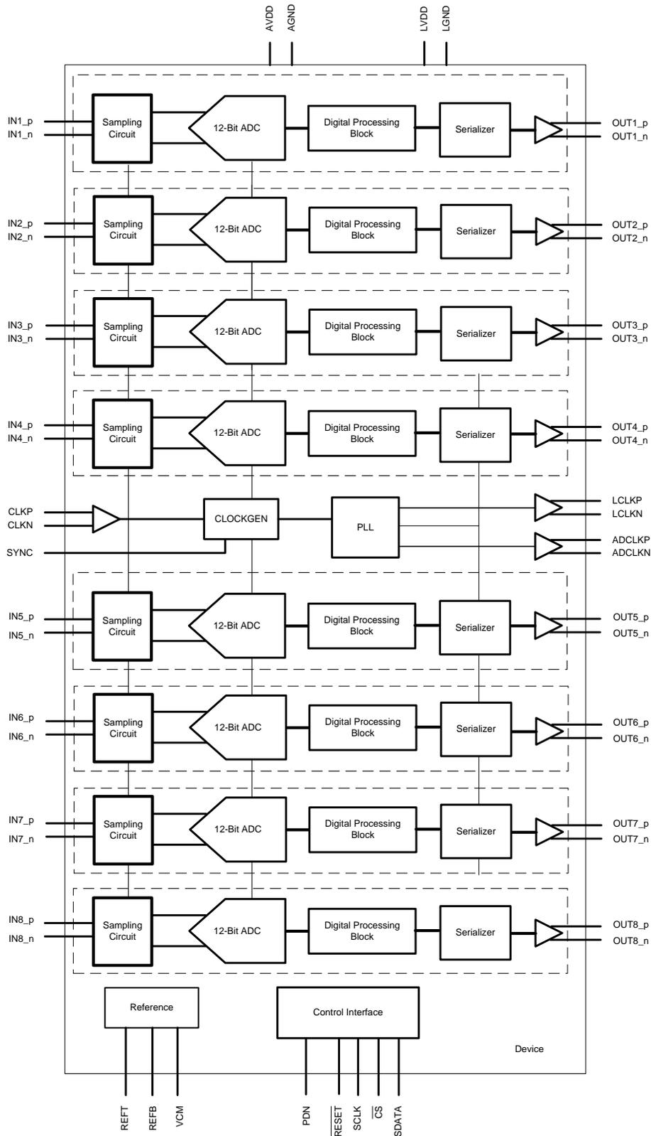
Figure 4. 10- and 12-Bit, 8-Channel ADC, Non-Interleaving Mode
