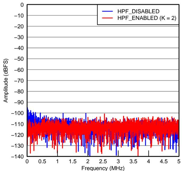
**Figure 33. FFT WITH HPF ENABLED AND DISABLED**
