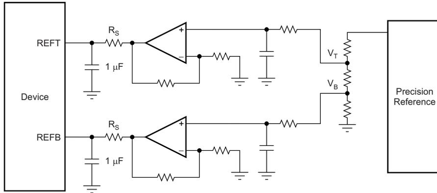
Figure 92. Driving Reference Inputs in External Reference Mode
