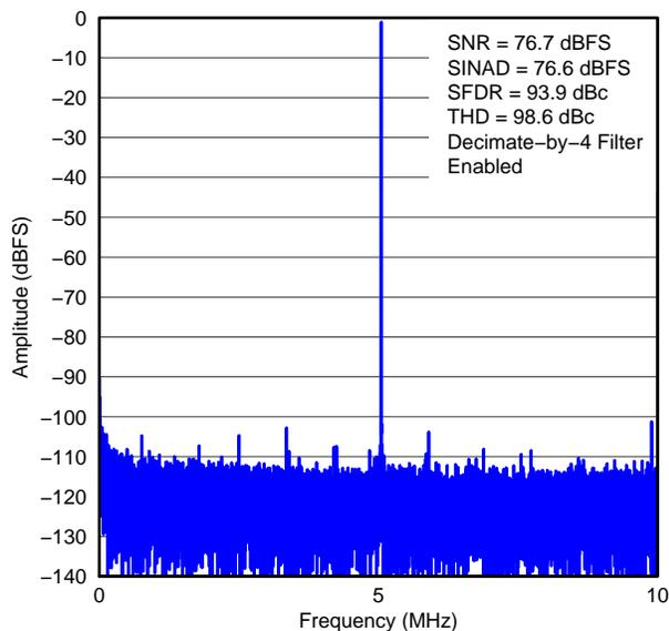
**Figure 30. FFT FOR 5-MHz INPUT SIGNAL**
