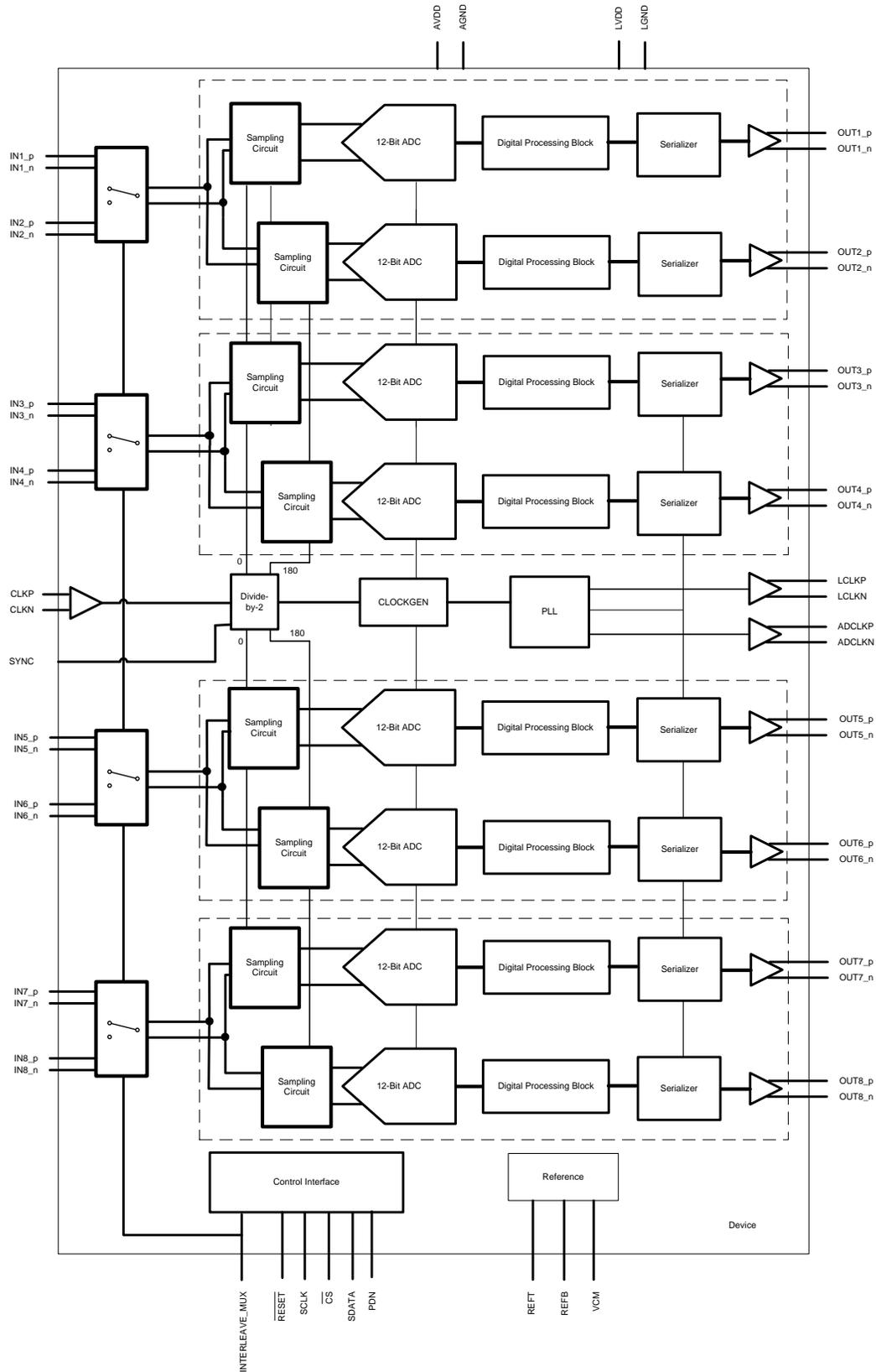
Figure 5. 10- and 12-Bit, 4-Channel ADC, Interleaving Mode
