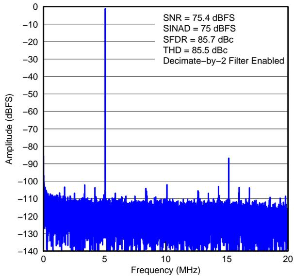
**Figure 28. FFT FOR 5-MHz INPUT SIGNAL (Sample Rate = 80 MSPS, Decimation Filter = 2) <sup>(1)</sup>**
