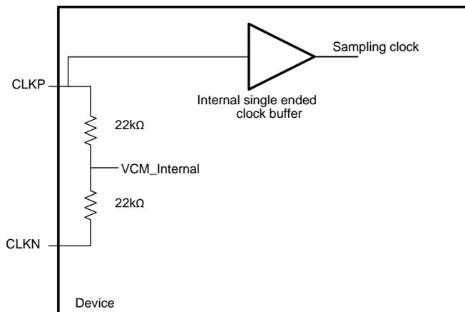
**Figure 89. Input Clock Equivalent Circuit: Single-Ended Mode**
