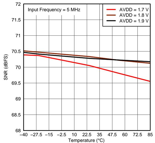
**Figure 21. SIGNAL-TO-NOISE RATIO vs AVDD AND TEMPERATURE**
