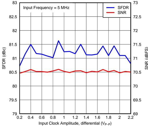
**Figure 18. PERFORMANCE vs INPUT CLOCK AMPLITUDE**
