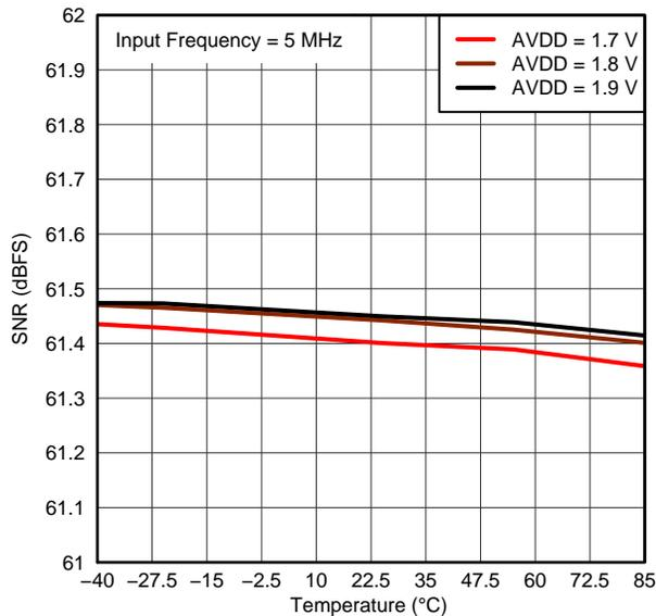
**Figure 51. SIGNAL-TO-NOISE RATIO vs AVDD AND TEMPERATURE**
