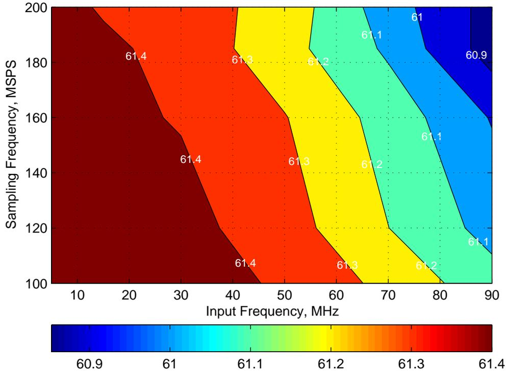
Figure 59. SIGNAL-TO-NOISE RATIO vs INPUT AND SAMPLING FREQUENCIES
