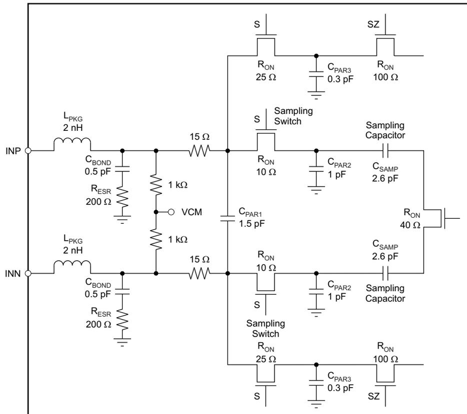
Figure 77. Analog Input Equivalent Circuit
