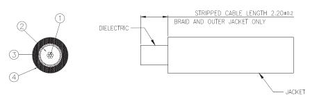
NOTE: JACKET STRIP OD DEFORMED MUST BE THAN LESS Ø3.30mm AFTER CUT OFF.
