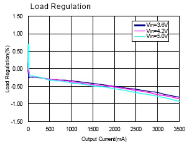
**Typical Performance Characteristics (cont.)** (@ $T_A = +25^\circ\text{C}$ ,  $C_{IN} = 10\mu\text{F}$ ,  $C_O = 10\mu\text{F}$ ,  $V_O = 1.2\text{V}$ , unless otherwise specified.)
