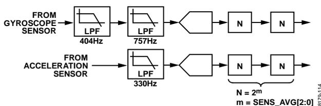
Figure 14. MEMS Analog and Digital Filters
