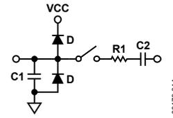
Figure 16. Equivalent Analog Input Circuit
