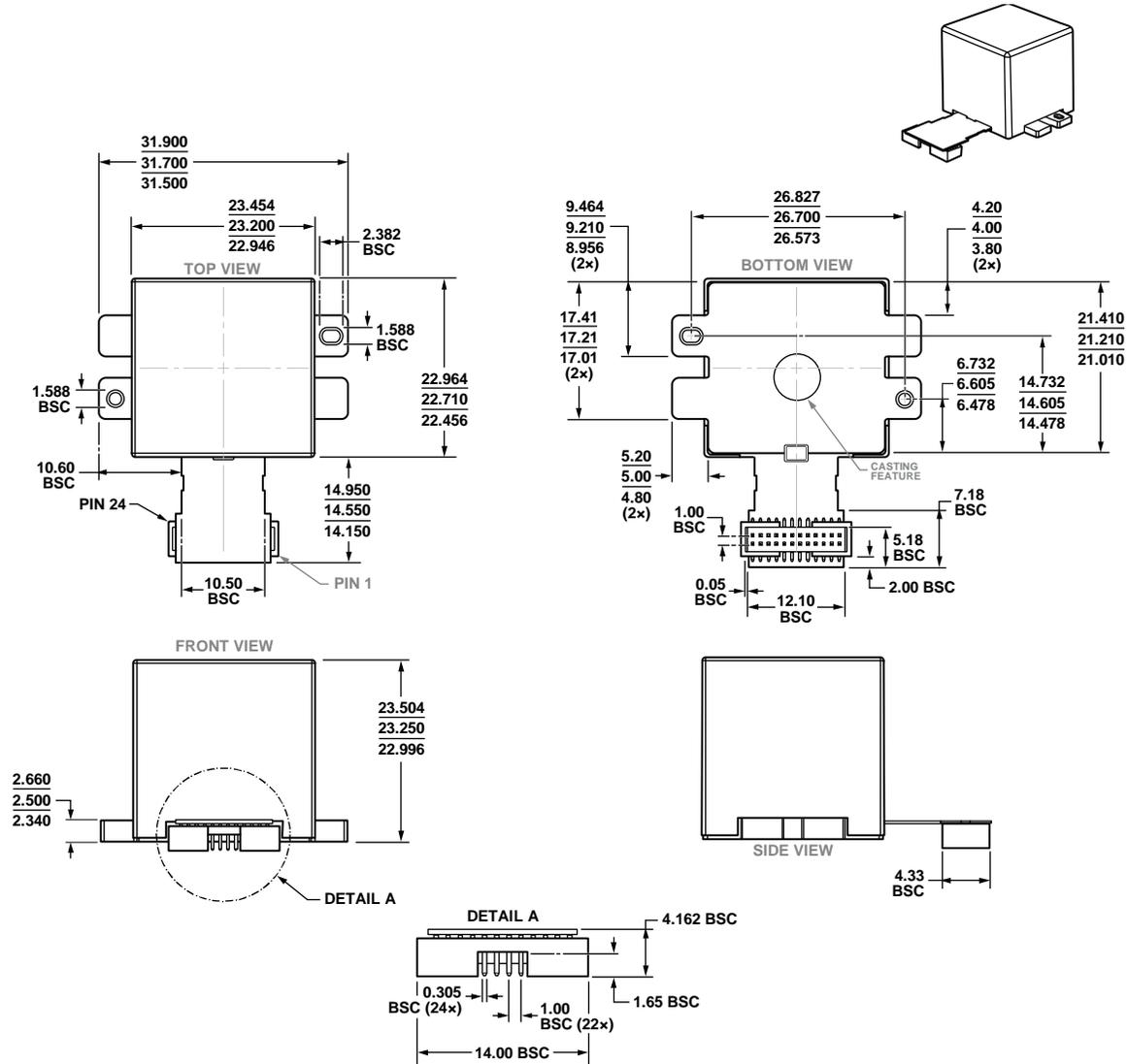
Figure 18. 24-Lead Module with Connector Interface (ML-24-2)
