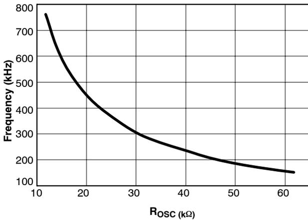
Figure 8. Switching Frequency
