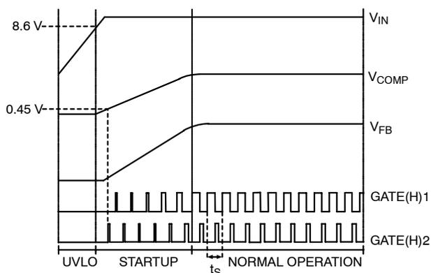
Figure 4. Idealized Waveforms
