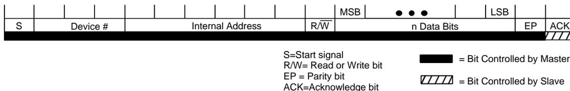
**Figure 10. Write Transaction, master write data to LM95010**
