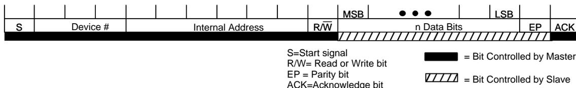
**Figure 9. Read Transaction, master reads data from LM95010**
