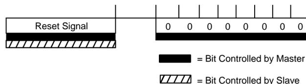
**Figure 8. Bus Reset Transaction**
