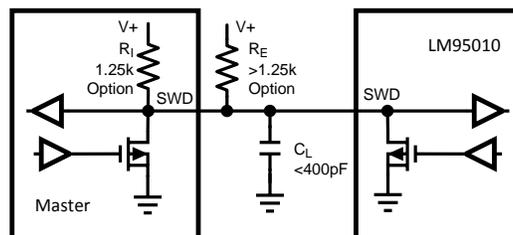
Figure 7. SensorPath SWD simplified schematic
