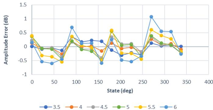
While the above shows amplitude error at particular frequencies vs phase shifter state, another common way to look at this parameter is error vs frequency.
