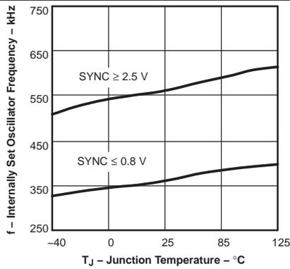
Figure 3. Internally Set Oscillator Frequency vs Junction Temperature
