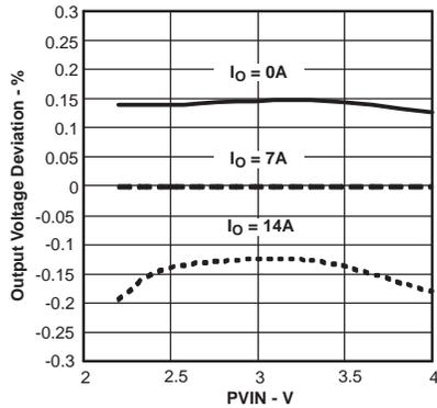
Figure 17. Line Regulation vs Input Voltage
