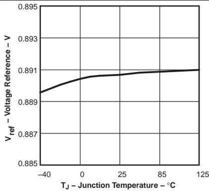
Figure 5. Voltage Reference vs Junction Temperature
