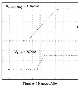
**Figure 32. Start-Up Waveform Output Voltage Relative to Enable**
