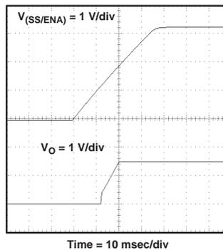
**Figure 22. Start-Up Waveform Output Voltage Relative To Enable**
