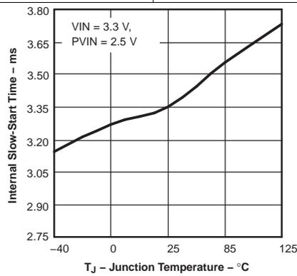
**Figure 9. Internal Slow-Start Time vs Junction Temperature**
