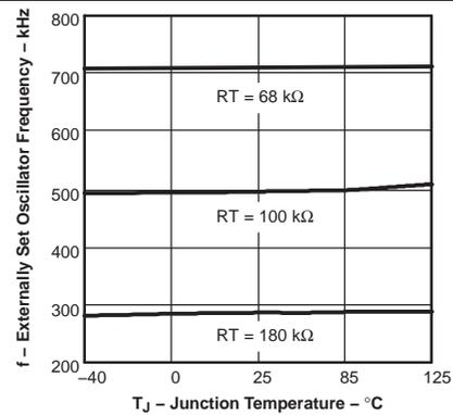
Figure 4. Externally Set Oscillator Frequency vs Junction Temperature
