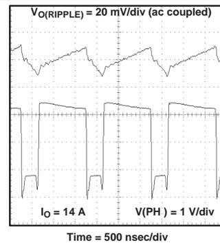
Figure 20. Output Voltage Ripple
