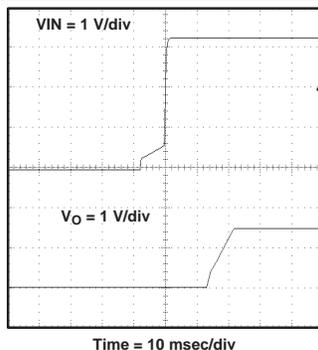
**Figure 23. Start-Up Waveform Output Voltage Relative To VIN**
