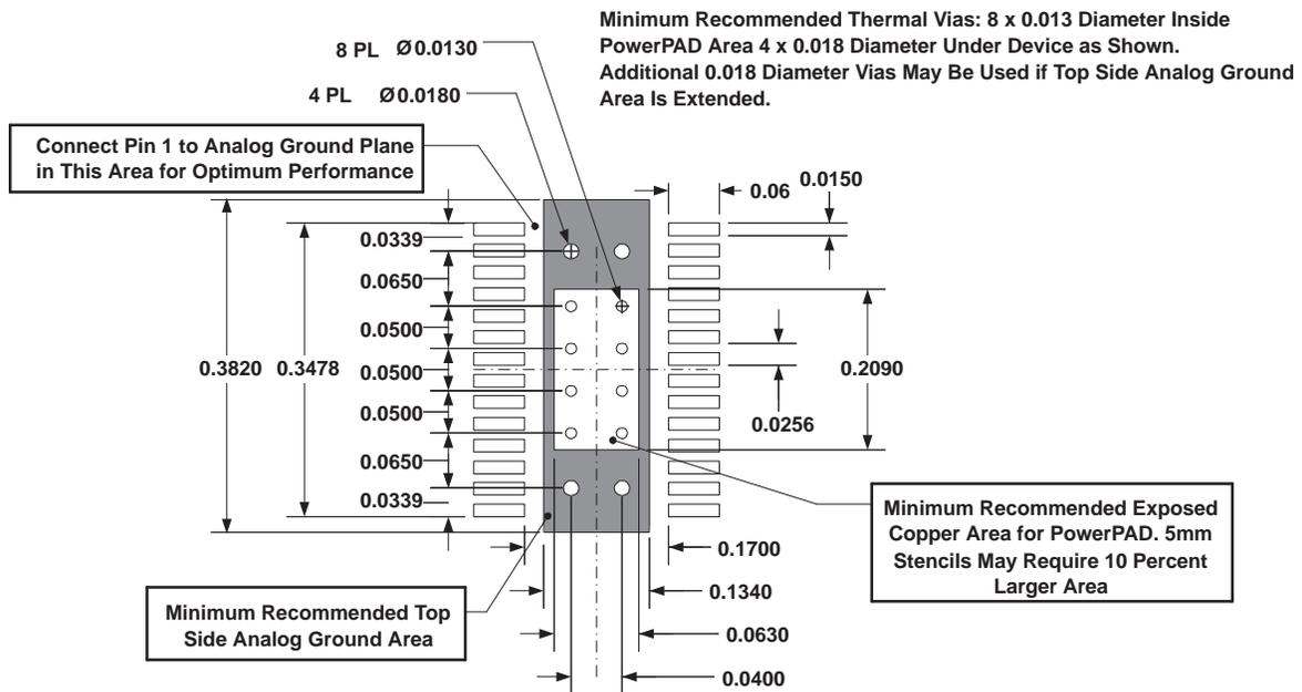
Figure 34. Recommended Land Pattern for 28-Pin PWP PowerPAD
