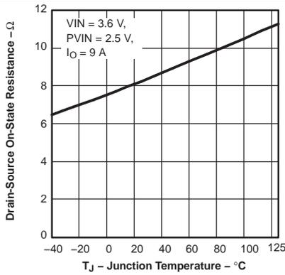
Figure 1. Drain-Source On-State Resistance vs Junction Temperature
