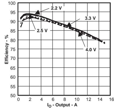
Figure 18. Efficiency vs Output Current
