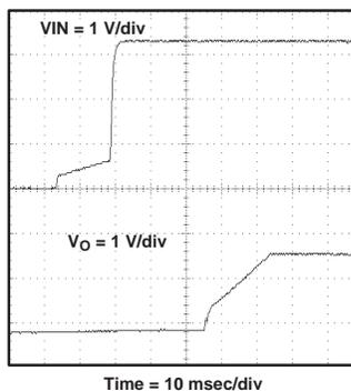
**Figure 33. Start-Up Waveform Output Voltage Relative to Enable**
