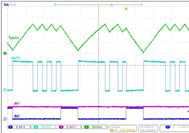
**Figure 12. Current Regulation With  $R_{ILIM} = 50.5\text{ k}\Omega$**
