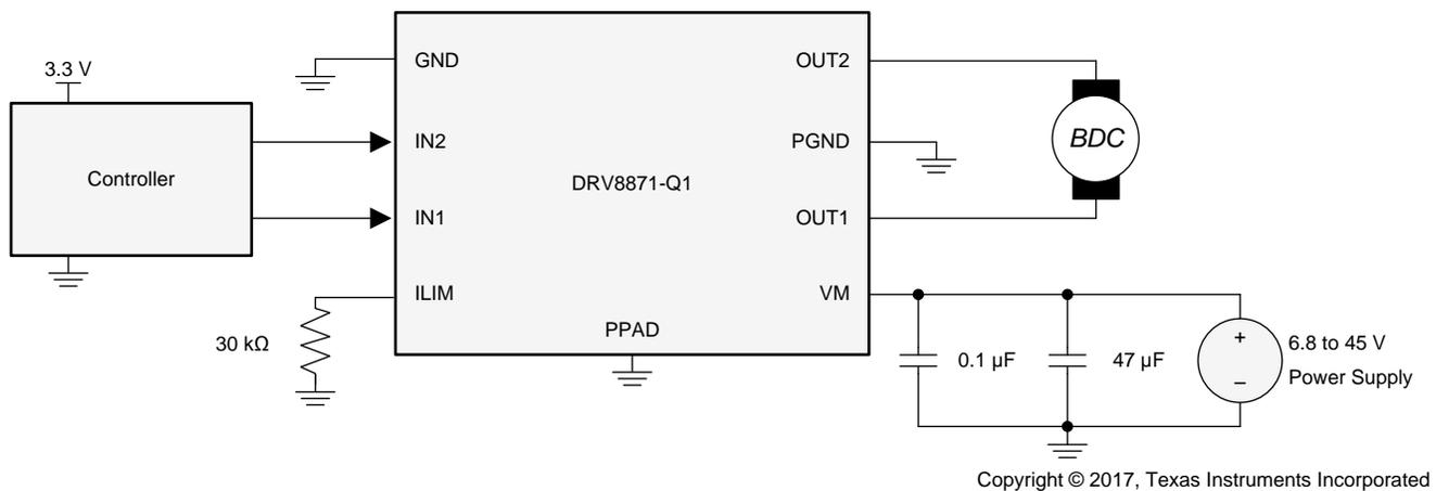
Figure 7. Typical Connections
