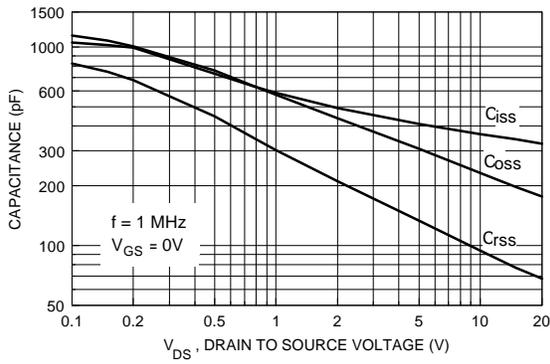
**Figure 9. Capacitance Characteristics.**
