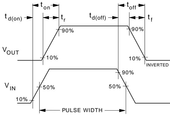
**Figure 12. Switching Waveforms.**
