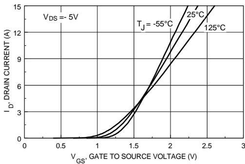
Figure 5. Transfer Characteristics.
