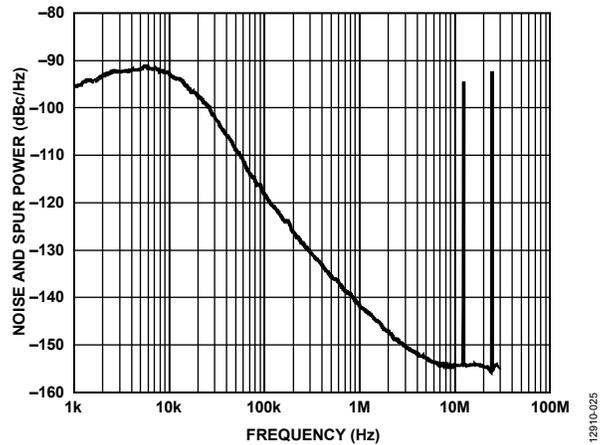
Figure 19. Fractional-N Spur Performance, W-CDMA Band,  $RF_{OUTA+} = 2113.5$  MHz,  $REF_{IN} = 122.88$  MHz, PFD = 61.44 MHz, Output Divide by 2 Selected, Loop Filter Bandwidth = 20 kHz, Channel Spacing = 20 kHz
