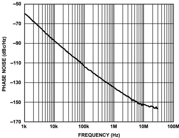
Figure 5. Open-Loop VCO Phase Noise, 5.0 GHz
