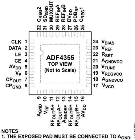
Figure 3. Pin Configuration
