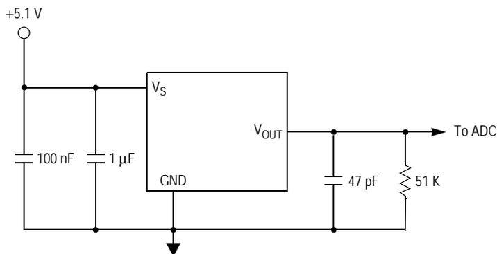
Figure 4. Typical application circuit (output source current operation)
