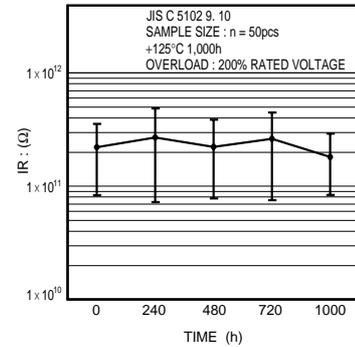
Fig.21 Insulation resistance
