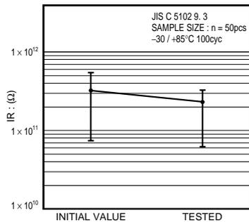
Fig.15 Insulation resistance
