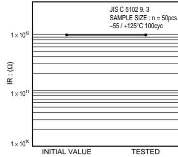
Fig.9 Insulation resistance
