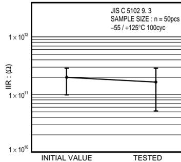
Fig.12 Insulation resistance
