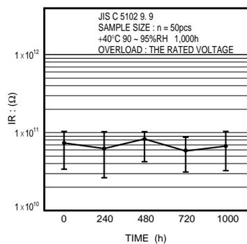
Fig.33 Insulation resistance
