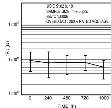
Fig.24 Insulation resistance
