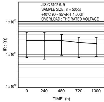
Fig.30 Insulation resistance
