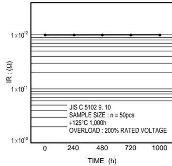
Fig.18 Insulation resistance
