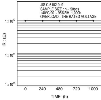
Fig.27 Insulation resistance
