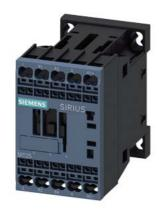
Power contactor, AC-3 9 A, 4 kW / 400 V 2 NO + 2 NC 24 V DC 4-pole Size S00 Spring-type terminals
