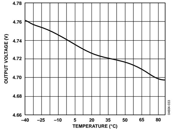
Figure 24. Receiver Output High Voltage vs. Temperature
