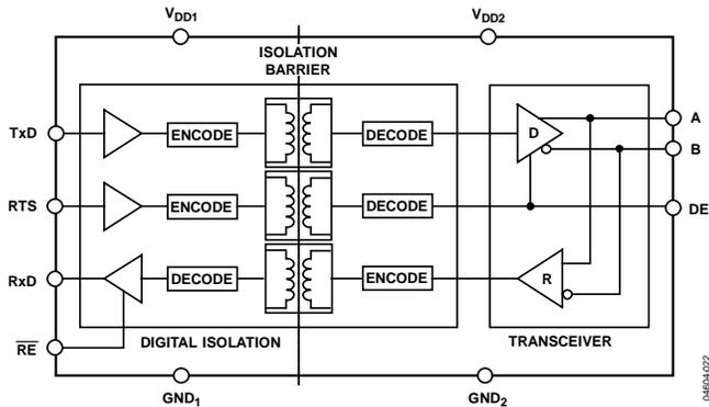
Figure 26. ADM2486 Digital Isolation and Transceiver Sections
