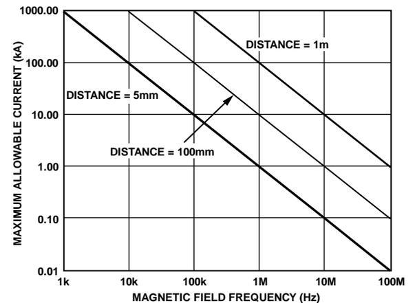
Figure 28. Maximum Allowable Current for Various Current-to-ADM2486 Spacings
