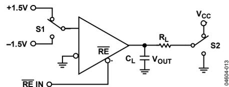
Figure 11. Receiver Enable/Disable
