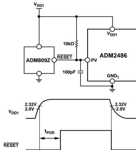
Figure 31. Driving PV with an Open-Drain Output
