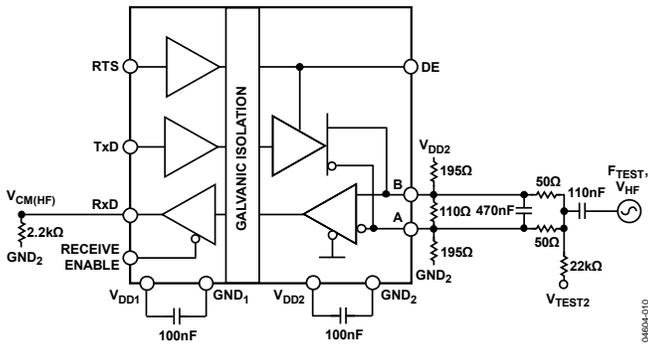
Figure 6. High Frequency Common-Mode Noise Test Circuit
