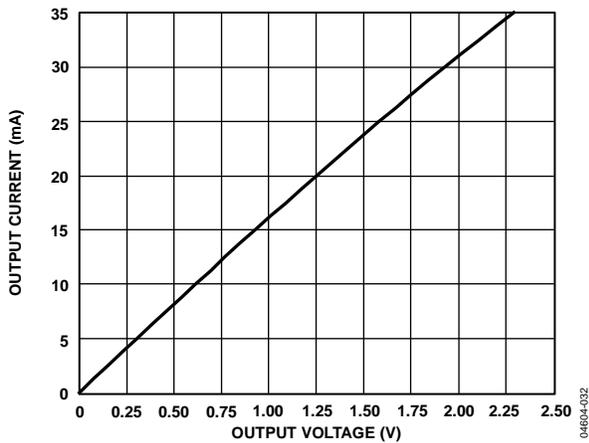
Figure 23. Output Current vs. Receiver Output Low Voltage
