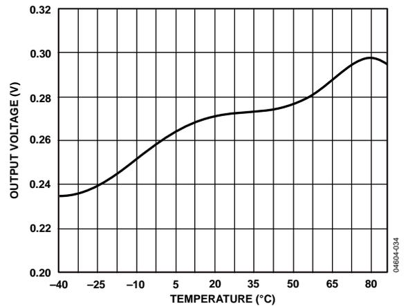
Figure 25. Receiver Output Low Voltage vs. Temperature
