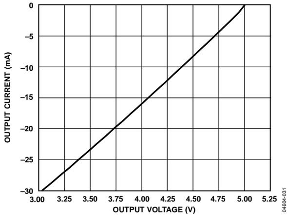
Figure 22. Output Current vs. Receiver Output High Voltage
