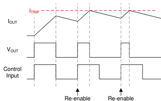
**Figure 7-4. Cycle-By-Cycle Current Regulation**
