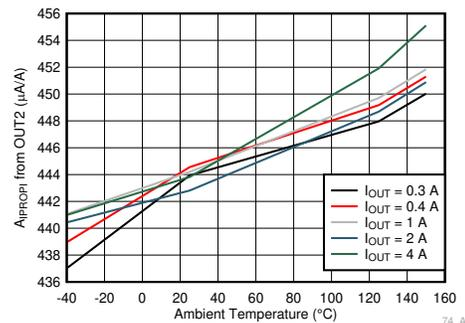
**Figure 6-9. OUT2 Current Sense Error vs. Junction Temperature**
