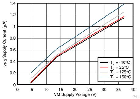
**Figure 6-2. Sleep Current ( $I_{VMQ}$ ) vs. Supply Voltage ( $V_{VM}$ )**
