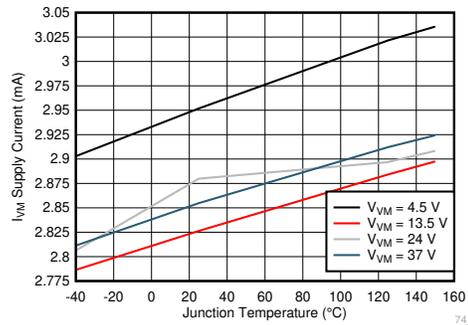
**Figure 6-5. Active Current ( $I_{VM}$ ) vs. Junction Temperature**
