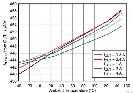
**Figure 6-8. OUT1 Current Sense Error vs. Junction Temperature**
