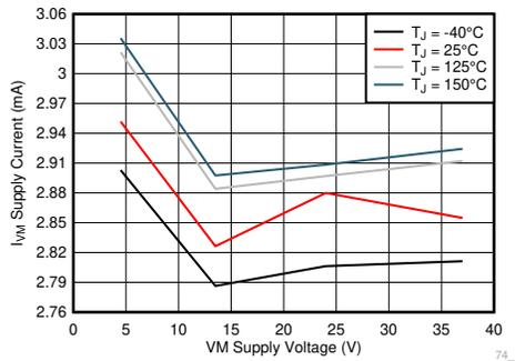
**Figure 6-4. Active Current ( $I_{VM}$ ) vs. Supply Voltage ( $V_{VM}$ )**
