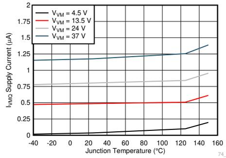
**Figure 6-3. Sleep Current ( $I_{VMQ}$ ) vs. Junction Temperature**
