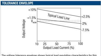
The voltage tolerance envelope shows typical load regulation characteristics for this product series. The tolerance envelope is the maximum output voltage variation due to changes in output loading.
