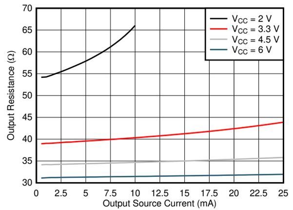
Figure 6-2. Output driver resistance in HIGH state.
