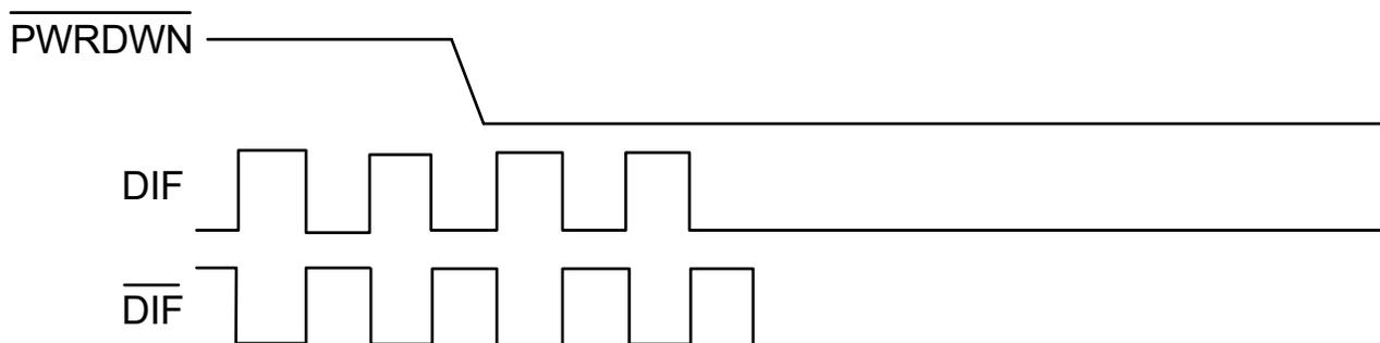
Figure 1.  $\overline{\text{PWRDN}}$  Assertion
