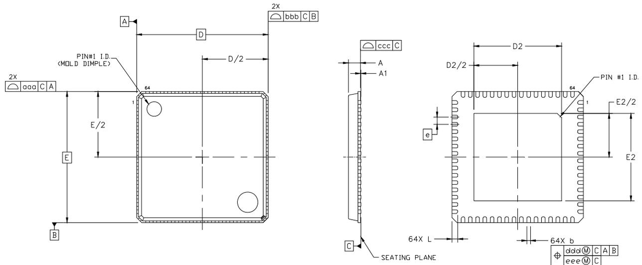
**Figure 13. 64-Pin Quad Flat No Lead (QFN) Package**
