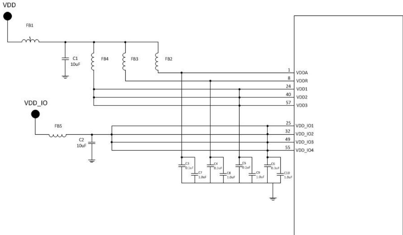
Figure 12. Schematic Example of Si53112 Power Filtering
